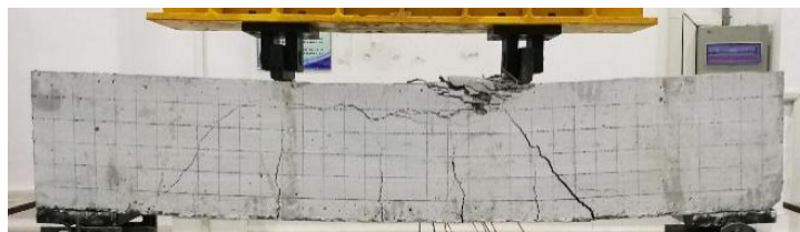
Figure5: Crack distribution of BS-1 beam
