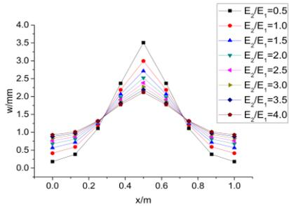
**Fig. 6.** Deflection of plate with different elastic modulus
