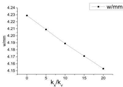
**Fig. 8.** Deflection of plate with different friction of A group
