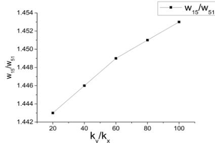
**Fig. 9.** Deflection of plate with different friction of B group
