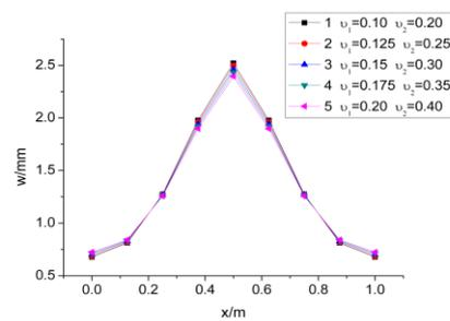
**Fig. 7.** Deflection of plate with different Poisson's ratio
