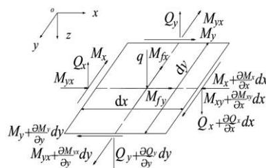
**Fig. 2.** Element of rectangular plate
