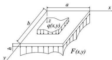
**Fig.1.** rectangular plate on Winkler elastic foundation
