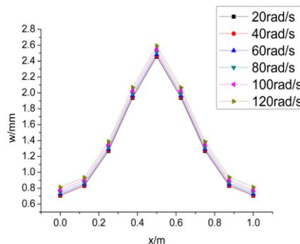
**Fig. 10.** Deflection of plate with different excitation frequency
