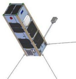
Fig. 3. 12U CubeSat (Aoxiang Zhixing)
