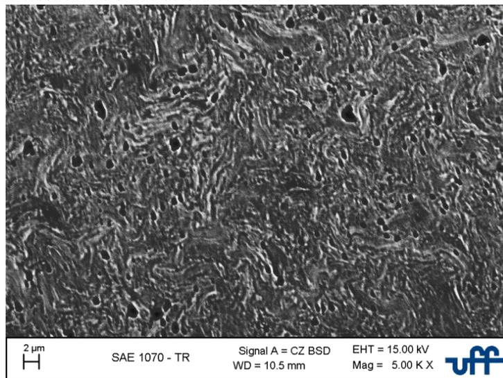
**Figure no1:** SEM. Cross section of SAE 1070 steel cold-deformed with accumulates strain of 2.52.
