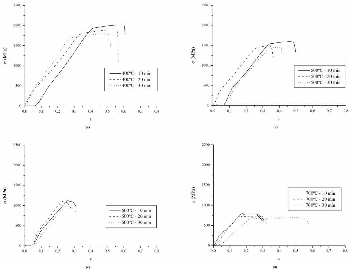
**Figure no 7:** Stress – strain curves of SAE 1070 steel annealed at (a) 400°C, (b) 500°C, (c) 600°C and (d) 700°C.
