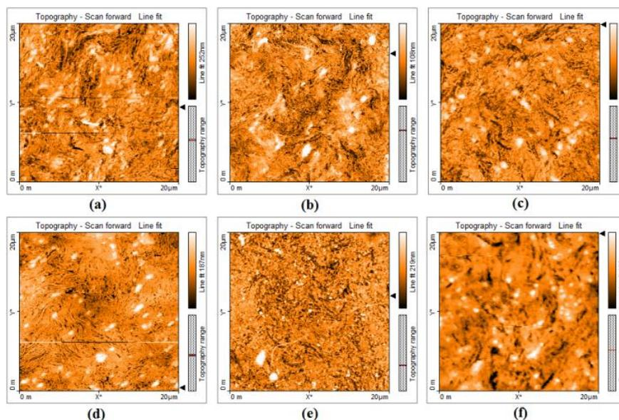
**Figure no 2:** AFM. Micrograph of SAE 1070 steel annealed at 400°C during (a) 5min, (b) 10min, (c) 15min, (d) 20min, (e) 25min, (f) 30min. Analyzed area of  $400 \mu\text{m}^2$ .
