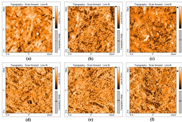
Figure no 4: AFM. Micrograph of SAE 1070 steel annealed at 600°C during (a) 5min, (b) 10min, (c) 15min, (d) 20min, (e) 25min, (f) 30min. Analyzed area of 400 µm<sup>2</sup>.
