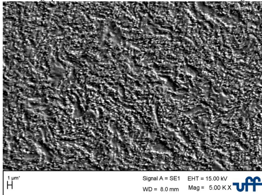
**Figure no 6:** SEM. Cross section of SAE 1070 steel annealed at 600°C for 30 min.
