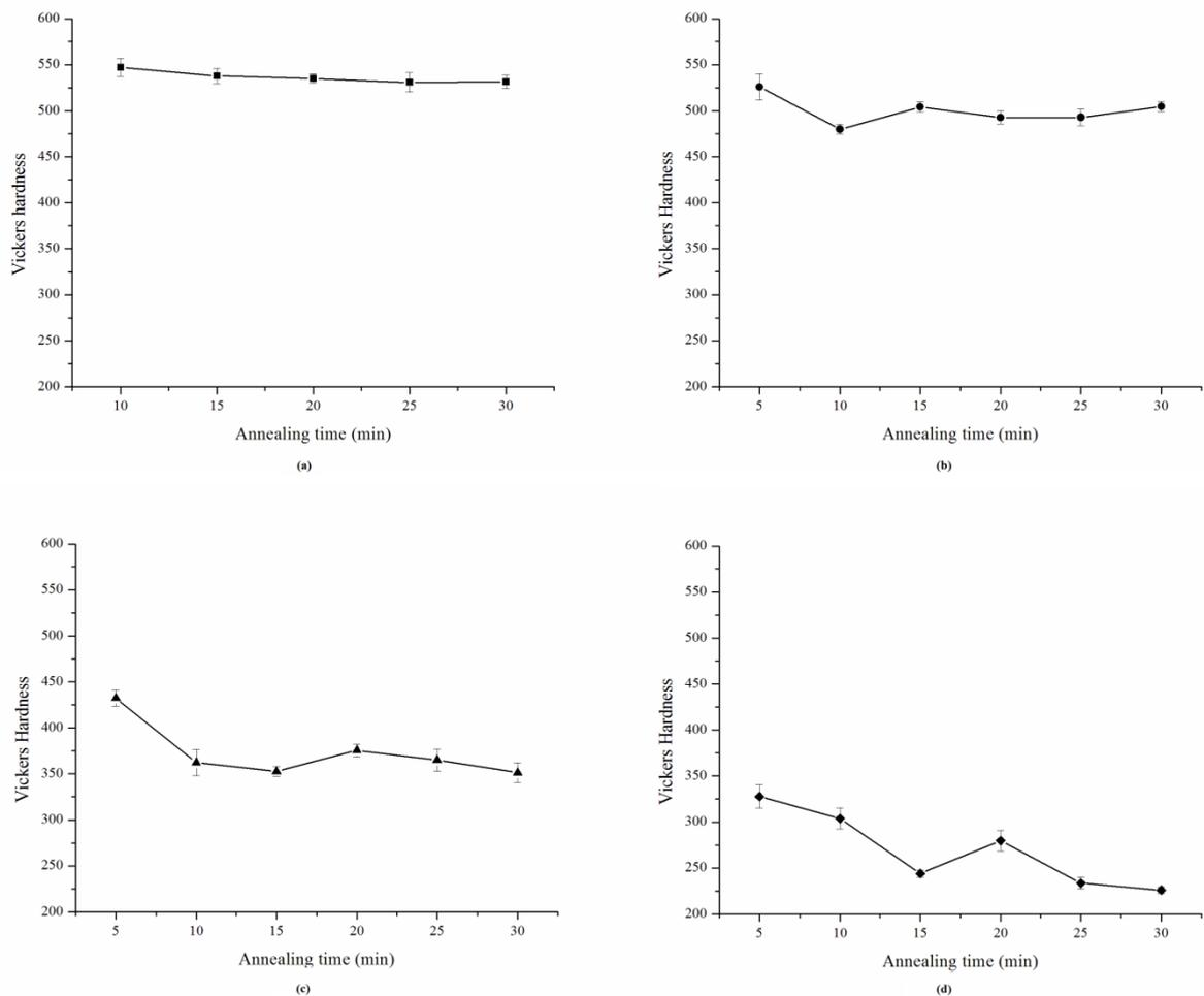
Figure no 8: SAE 1070 Vickers Hardness evolution annealed at (a) 400°C, (b) 500°C, (c) 600°C and (d) 700°C
