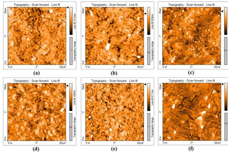
Figure no 3: AFM. Micrograph of SAE 1070 steel annealed at 500°C during (a) 5min, (b) 10min, (c) 15min, (d) 20min, (e) 25min, (f) 30min. Analyzed area of 400 µm<sup>2</sup>.
