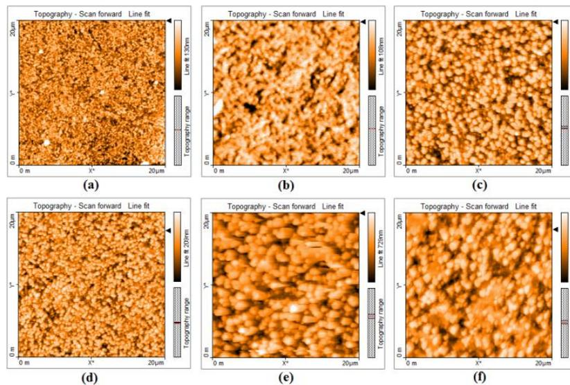
Figure no 5: AFM. Micrograph of SAE 1070 steel annealed at 700°C during (a) 5min, (b) 10min, (c) 15min, (d) 20min, (e) 25min, (f) 30min. Analyzed area of 400 µm<sup>2</sup>.
