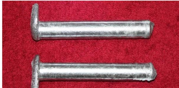
**Figure 1:** Prepared LM29-B<sub>4</sub>C composites
