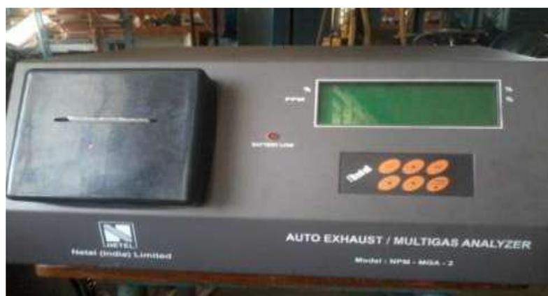
Fig 4.2: Gas Analyzer
