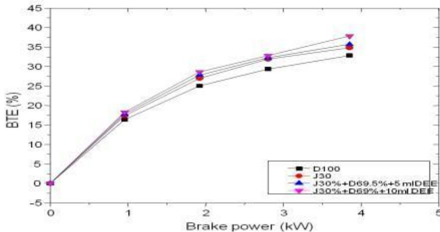
**Fig.5.1** Variation of Brake thermal efficiency with brake power
