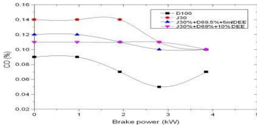
Fig.5.4 Variation of Carbon monoxide with brake power
