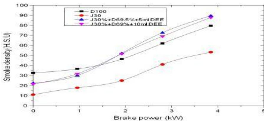
Fig.5.3 Variation of Smoke density with brake power
