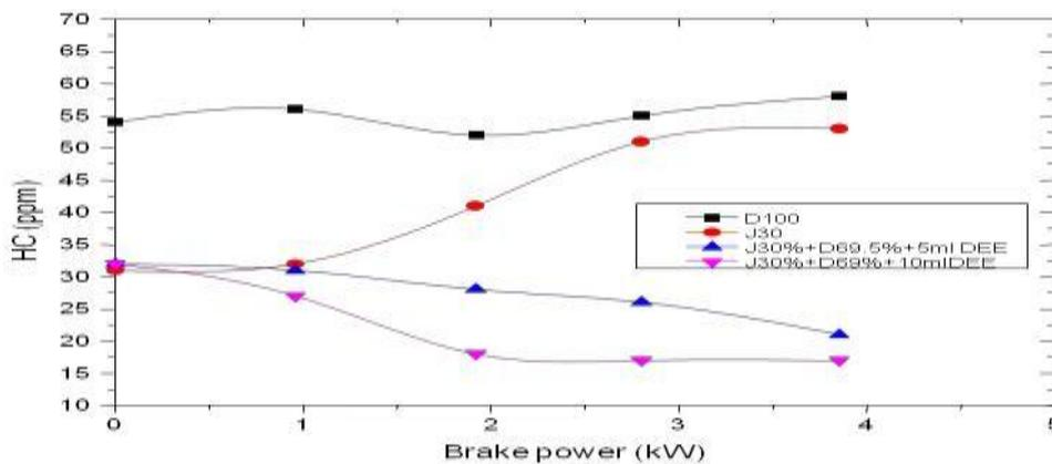
Fig.5.5 Variation of unburned hydrocarbons with brake power
