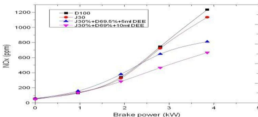
Fig 5.6 Variation of NO<sub>x</sub> with brake power
