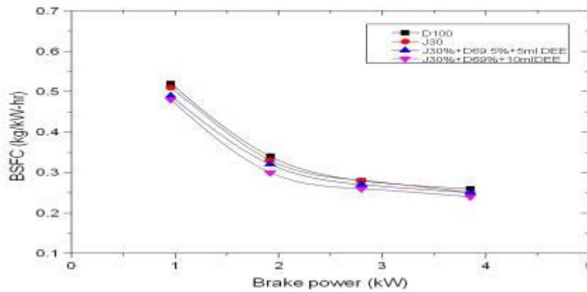
Fig.5.2 Variation of BSFC with brake power
