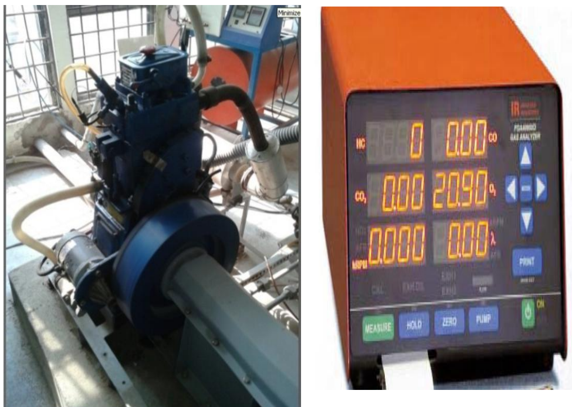
Fig.3 Single cylinder, four stroke, multi-fuel, research engine connected to eddy type dynamometer and DC five gas analyzer.
