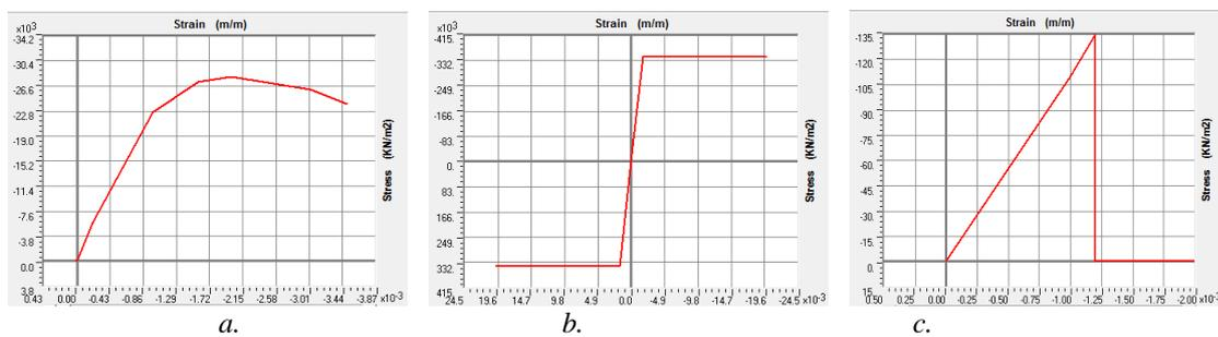
Fig. 2 – The stress-strain curves: a. concrete; b. steel; c. masonry
