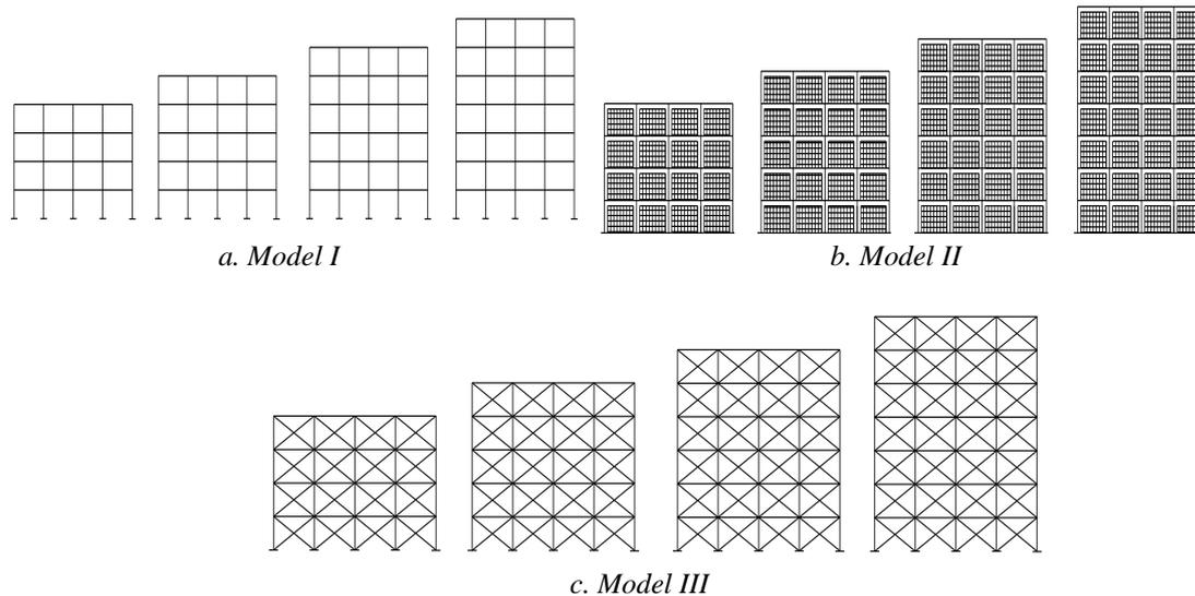
Fig. 1 – Different cases of masonry infill frames
