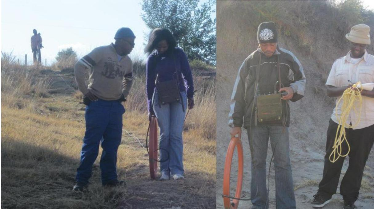
Figure 4 Electromagnetic survey using EM34-3 terrain conductivity meter.
