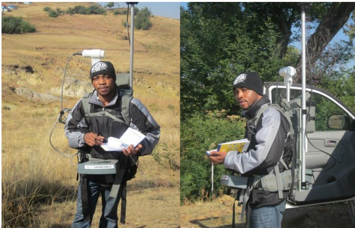
Figure 3 Magnetic survey using G-859SX portable caesium vapor magnetometer.
