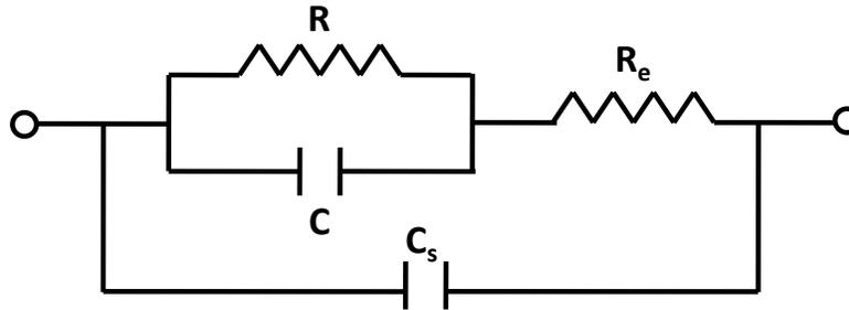
Figure 3: Soil electrical equivalent circuit considering electrode resistance and stray capacitance [27]
