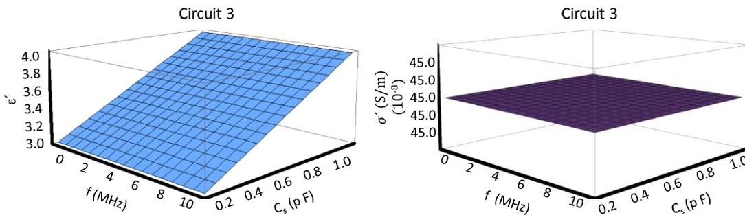
Figure 6: (a) Plot of real relative permittivity vs. stray capacitance and (b) plot of conductivity vs. stray capacitance for circuit 3
