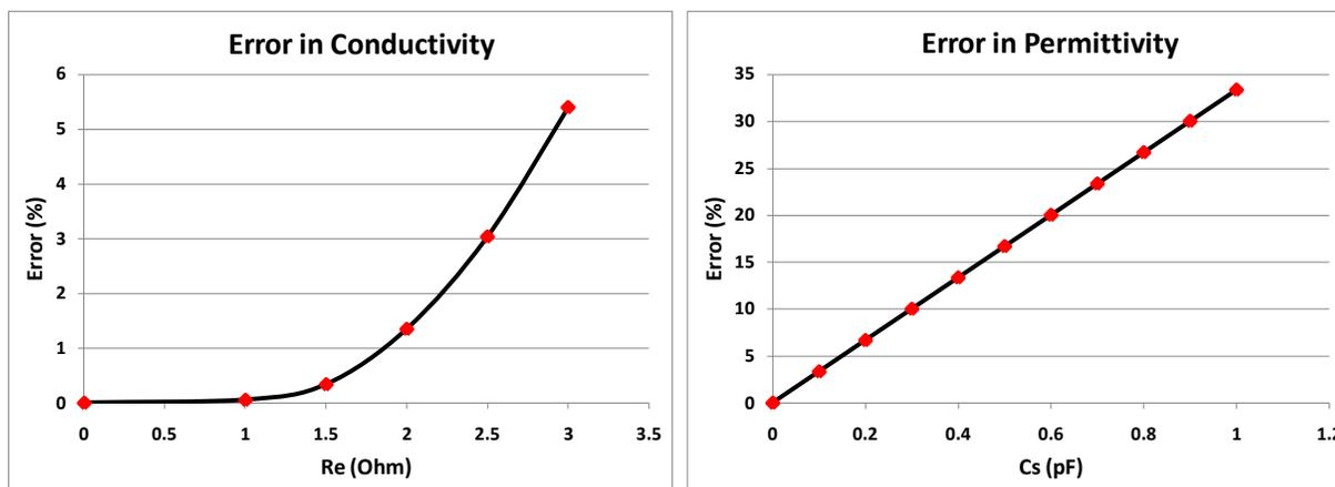
Figure 7: (a) Error in conductivity due to electrode resistance and (b) error in permittivity due to  $\epsilon_s$  capacitance
