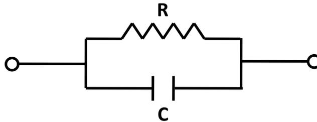
Figure 1: Simplest soil electrical equivalent circuit 1 [21, 22]
