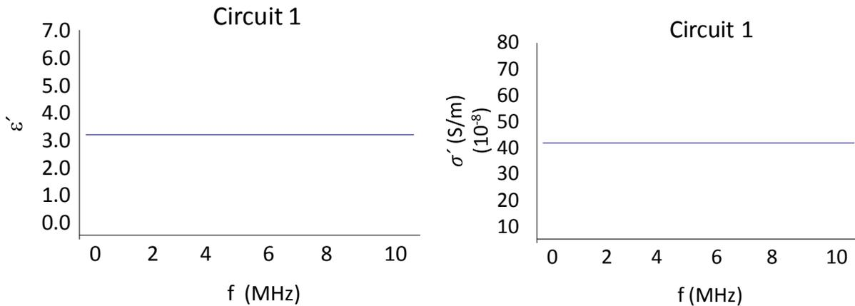
Figure 4: (a) Plot of real relative permittivity vs. frequency and (b) plot of conductivity vs. frequency for circuit 1
