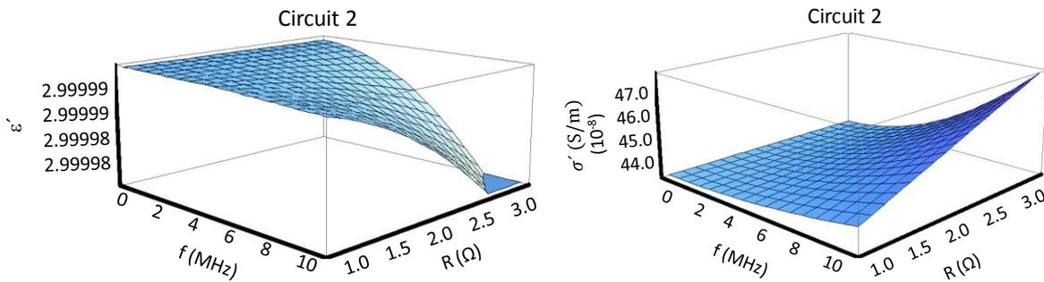
Figure 5: (a) Plot of real relative permittivity vs. electrode resistance and (b) plot of conductivity vs. electrode resistance for circuit 2
