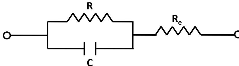
Figure 1: Soil electrical equivalent circuit 2 with electrode resistance included [24-25]
