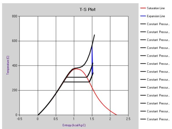
Fig.2 T-S Diagram for ST-1
