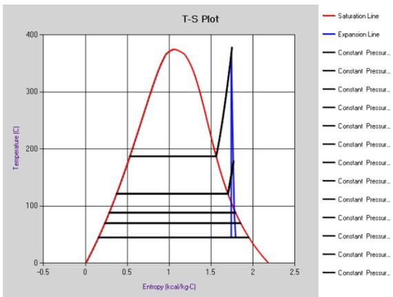
Fig.5 T-S Diagram for ST-4
