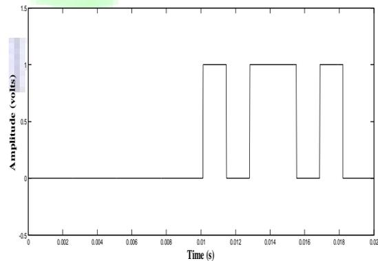
Fig.4c.Gating pattern of Switch (T<sub>12</sub>)
