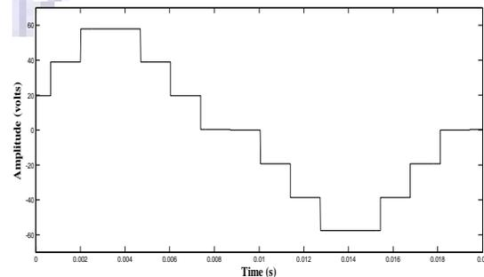
Fig.5c Seven level output of inverter
