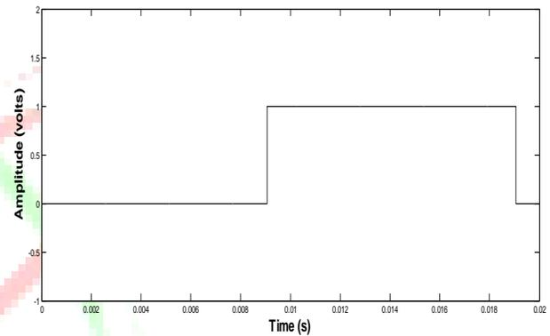
Fig.4b.Gating pattern of Switch (T<sub>13</sub>, T<sub>23</sub>)
