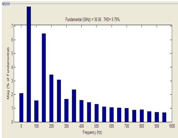
Fig.5d FFT analysis of load voltage for seven-level inverter
