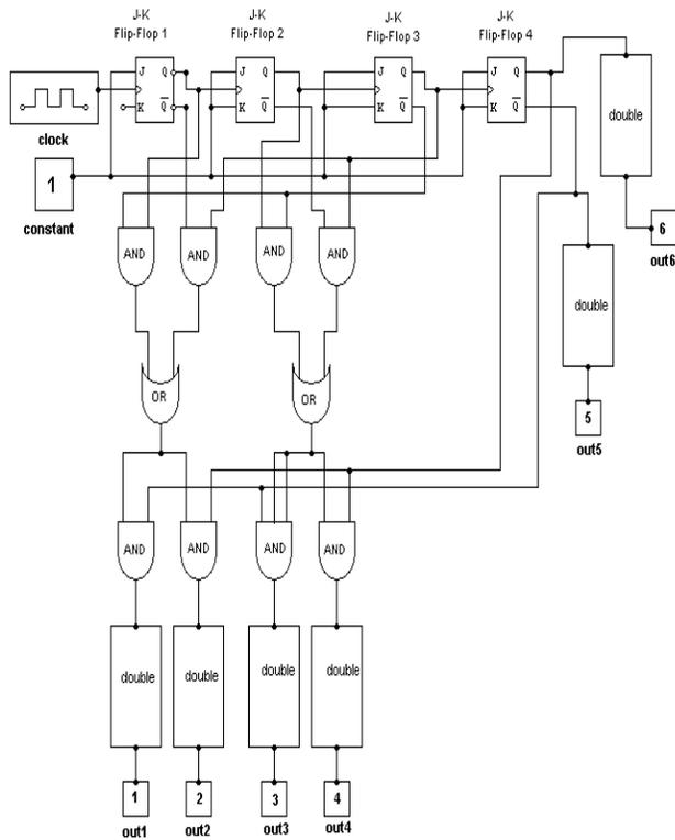
Fig.2 Firing circuit
