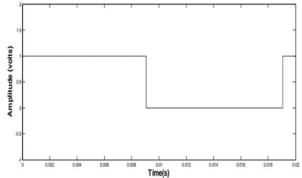
Fig.4a.Gating pattern of Switches (T<sub>11</sub>, T<sub>21</sub>)
