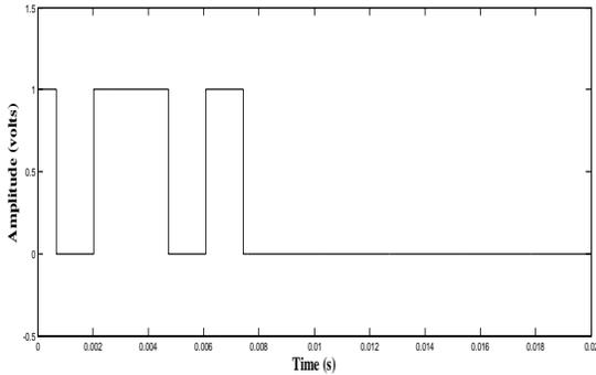
Fig.4d. Gating pattern of Switch ( $T_{14}$ )
