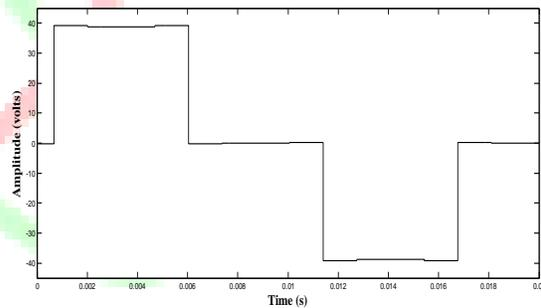
Fig.5b Output of Inverter 2.
