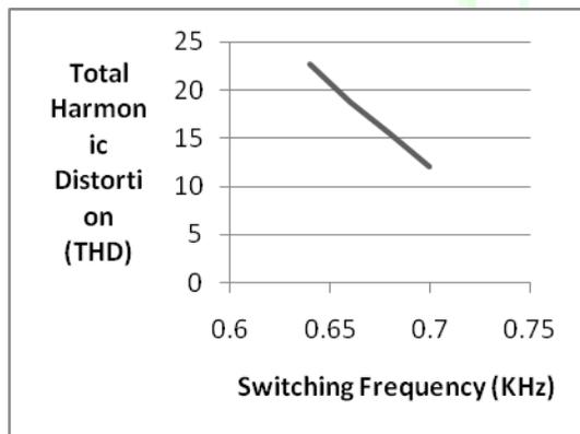
Fig.6 Switching Frequency Vs THD
