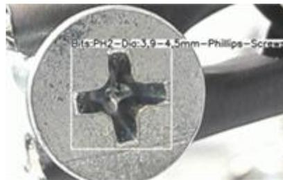
**Figure 3.2:** Correct identification of Phillips screw drive of bit size 2 with YOLOv8 [28]
