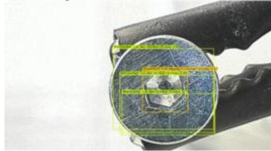
**Figure 3.5:** Wrong identification due to several classes with YOLOv8 [28]
