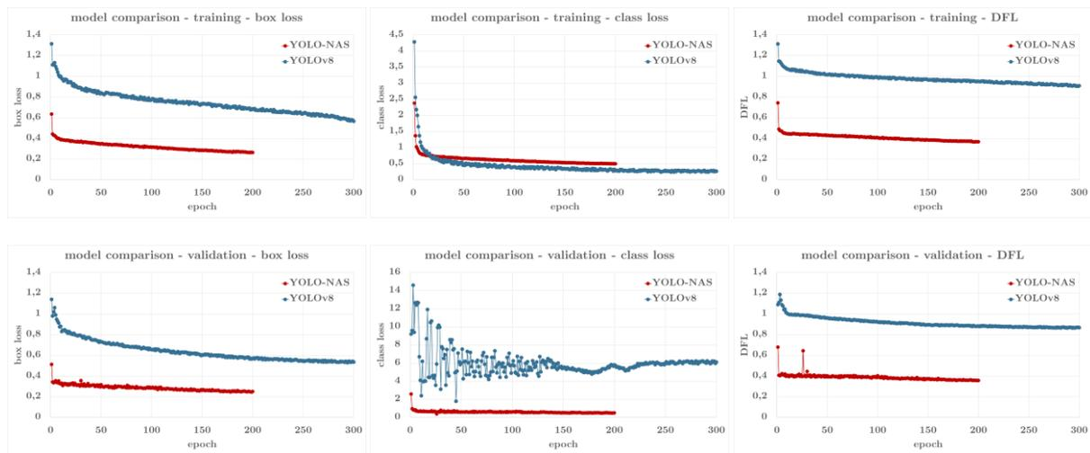
**Figure 2.4:** Training (top) and validation (bottom) loss curves for YOLO- NAS (red) and YOLOv8 (blue). From left to right: box loss, class loss, DFL [28]
