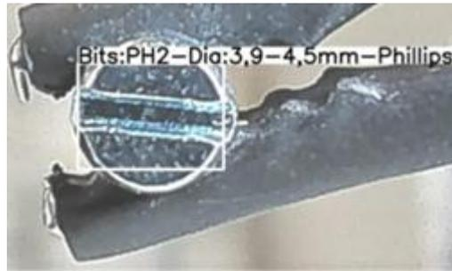
**Figure 3.3:** Wrong identification of Slotted 0.8 as Phillips PH2 with YOLOv8 [28]
