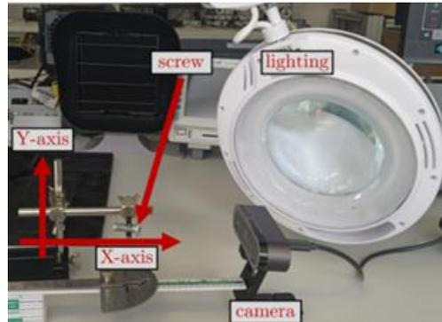
**Figure 3.6:** Experimental test setup of the screw in front of the camera along with a measuring scale, protractor, vice and lighting [28]
