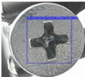
**Figure 3.1:** Correct identification of Phillips screw drive of bit size 2 with YOLO- NAS [28]
