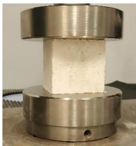
Image (32 ) shows the compression test of cubes Sample1(5 cm3)
