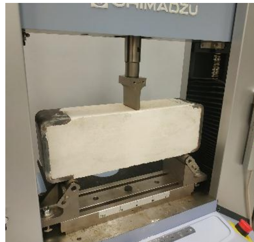
Image ( 40) shows loading pin before testing
