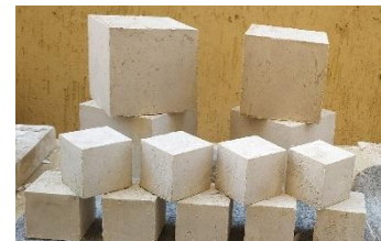
Image (28) shows the completion of casting the sample 10 cm 3 , 5 cm 3
