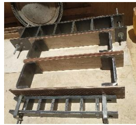
Image (24) shows preparing molds for casting
