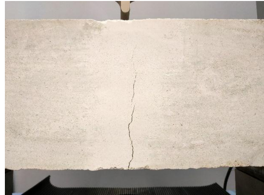
Image (24 ) showing the collapse of the mock-up
