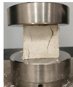
Image ( 35) shows the collapse of sample No. 2 after salt aging and in a wet condition
