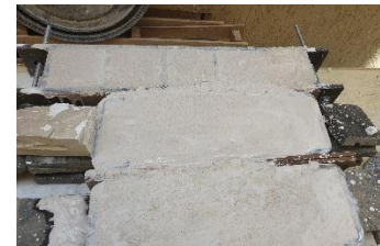
Image (25) shows the samples after pouring into the molds
