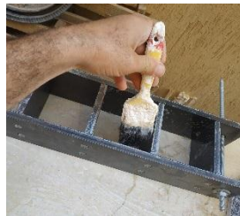
Image (23) shows the insulation of a 10 cm 3 sample casting mold
