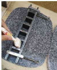
Image (22) shows the insulation of a 5 cm 3 sample casting mold
