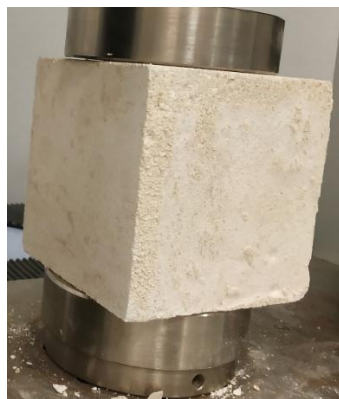
Image ( 36) shows the compression test of cubes Sample 3 (10 cm 3 )
