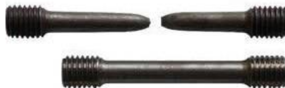
Figure 5: Tensile Test Specimen
