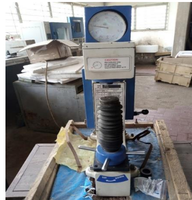
Figure 4: Brinell hardness Testing Machine
