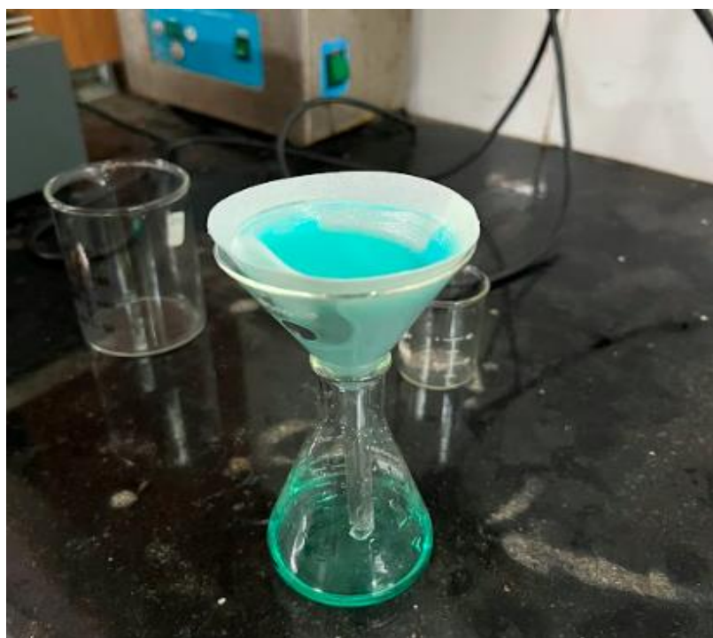
Fig. 1.1 - Filtration for preparation of precursor solution
