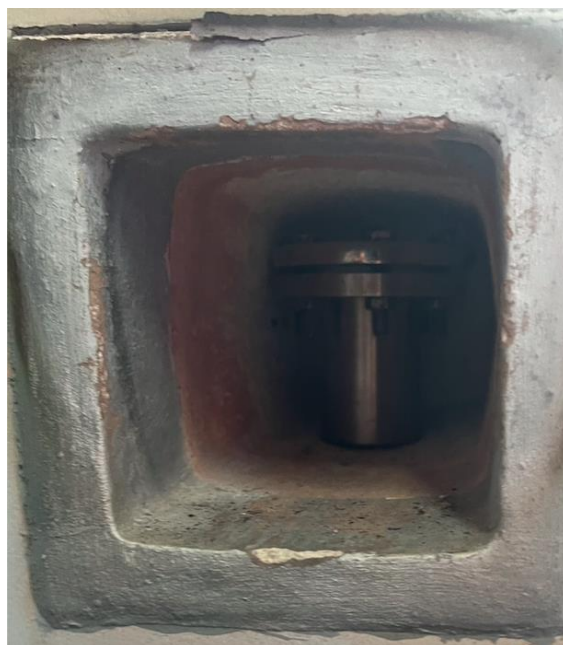
Fig. 1.2 - Autoclave inside muffle furnace
