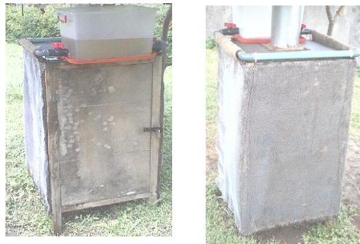
Plate 3: The cooling sub-system.
