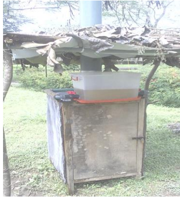
Plate 5: The experimental set-up showing the wind-powered evaporative cooler under a shed.
