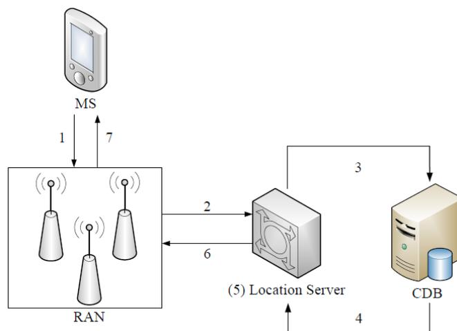
Figure 2: Diagram of RF fingerprinting location.
