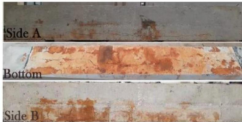
**Fig. 3.** Corrosion-induced cracks in beam PCB4
