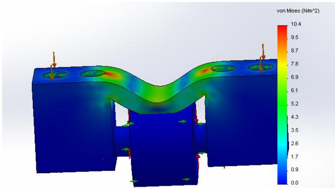
Figure 4.4 von mises stress value for the castor wheel
