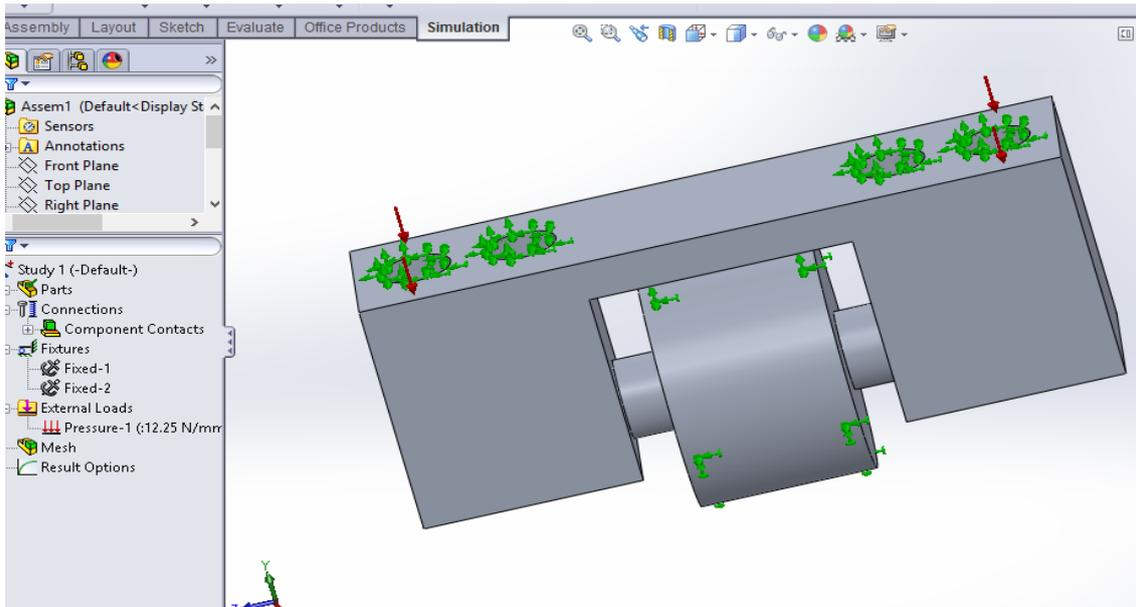
Figure 4.3 Applied pressure on the castor wheel as a result of user load
