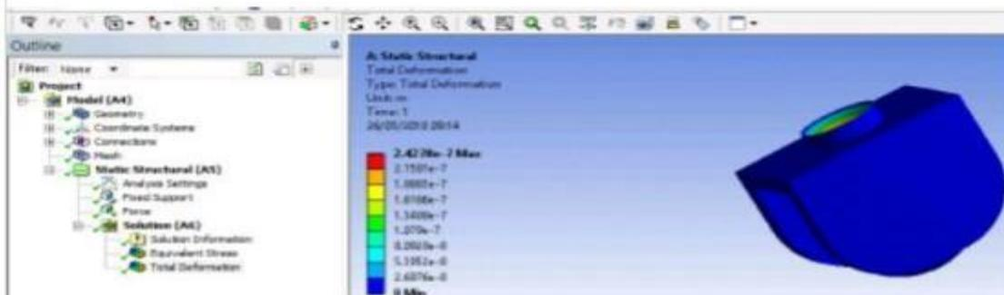
Maximum deformation =  $2.42 \times 10^{-7} \text{ m}$
