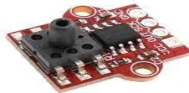
Figure 2: Pressure Sensor
