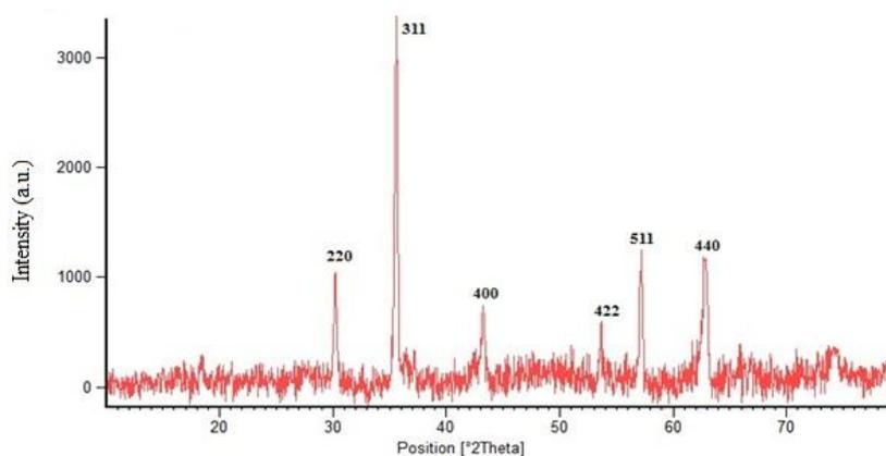
Figure 2: XRD pattern of chloride-CoFe<sub>2</sub>O<sub>4</sub>@PANI composite
