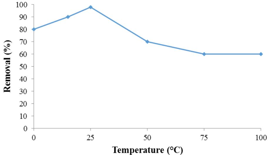
Figure (7): Investigation of the effect of temperature on removal
