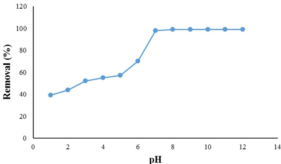
Figure 4: Effect of pH change on lead removal
