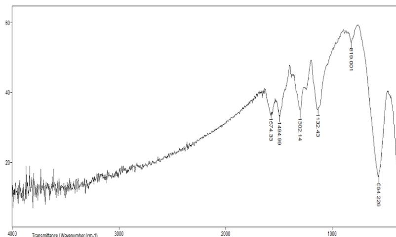
Figure 1: FT-IR spectrum of chloride -CoFe<sub>2</sub>O<sub>4</sub>@PANI Nanocomposite
