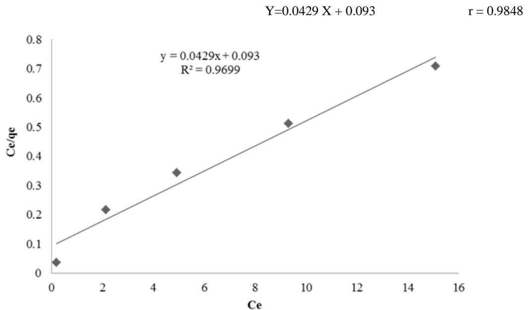
Figure 8: Langmuir curve
