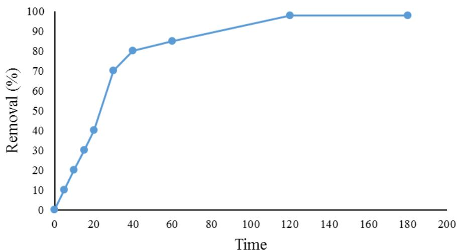
Figure 5: Effect of stirring time of adsorbent and lead solution
