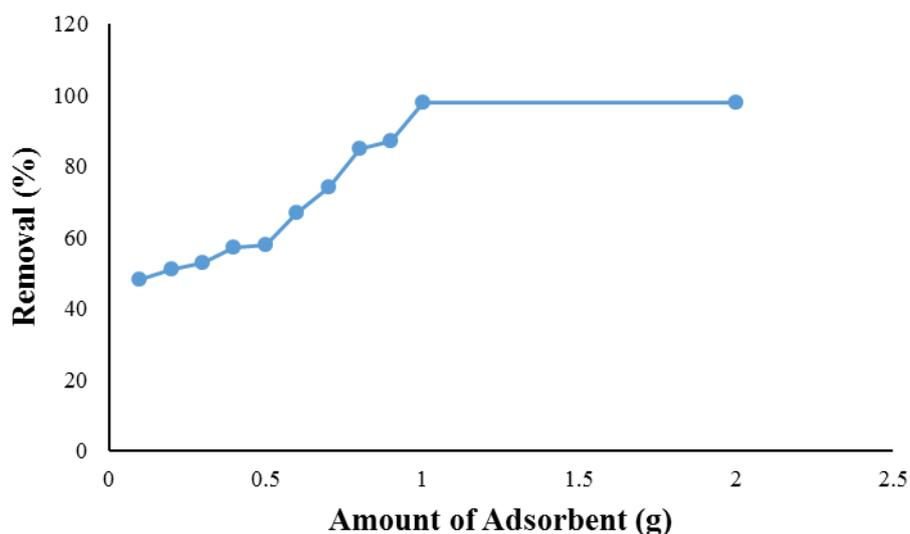
Figure 6: Effect of adsorbent amount on lead removal
