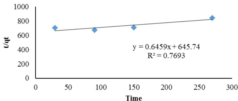
Figure 11: Investigation of a quasi-second order kinetic model
