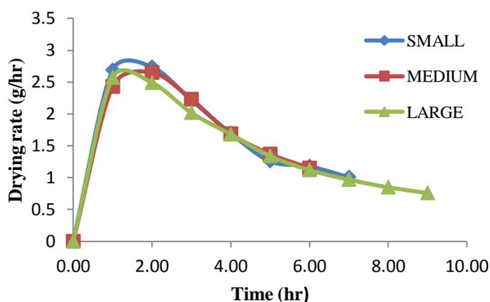
Figure 9: drying rate against drying time for the different size ranges of *Gnetum africanum*
