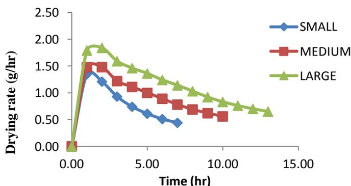
Figure 15: drying rate against drying time for the different size ranges of carrot
