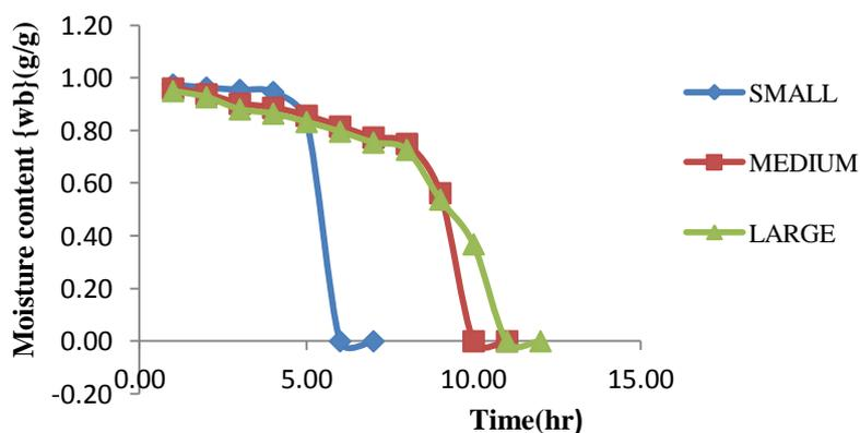
Figure 1: moisture content variation against time of drying different size ranges of spear grass vegetable
