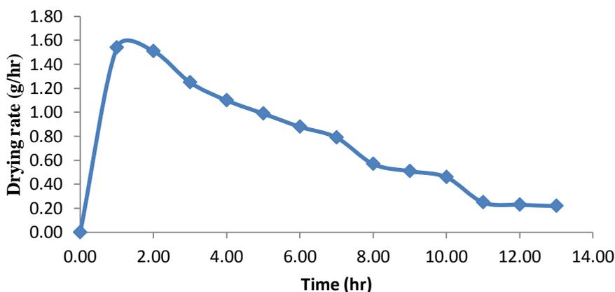
Figure 16: drying rate against drying time for bulk carrot
