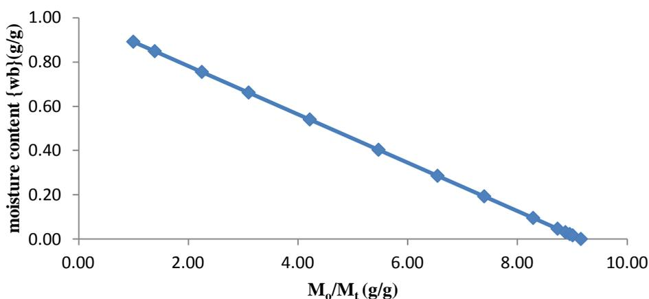
Figure 18: moisture content against  $M_o/M_t$  for bulk carrot
