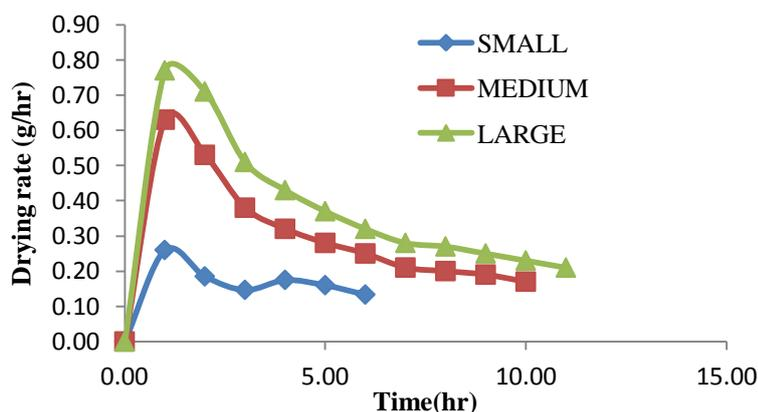
Figure 3: drying rate against drying time for the different size ranges of spear grass vegetable
