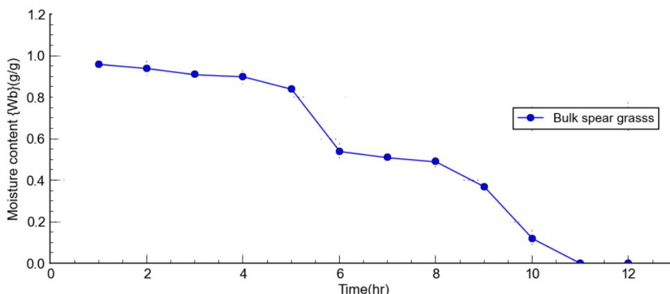
Figure 2: moisture content variation against time of drying the bulk of spear grass vegetable
