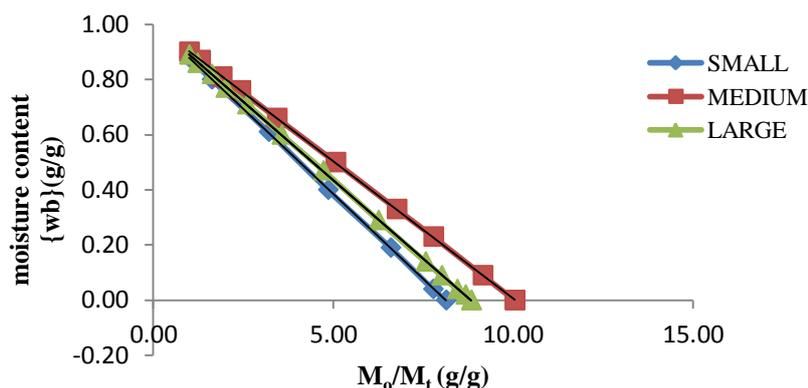
Figure 17: moisture content against  $M_o/M_t$  for the different size ranges of carrot
