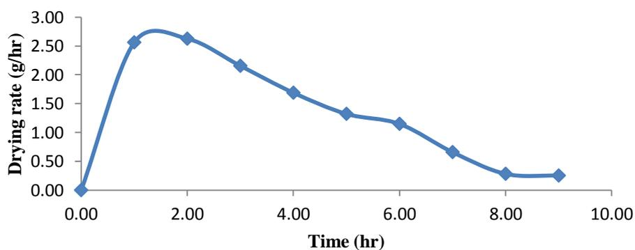
Figure 10: drying rate against drying time for bulk *Gnetum africanum*
