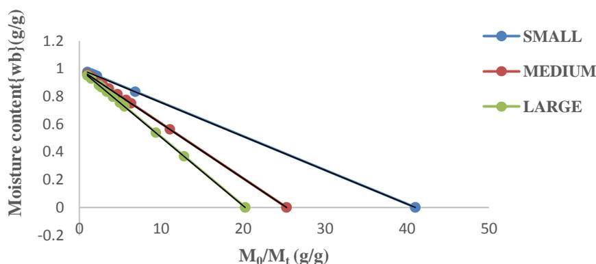
Figure 5: moisture content against  $M_0/M_t$  for the different size ranges of spear grass vegetable
