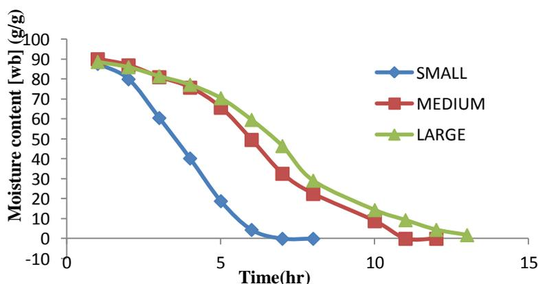
Figure 13: moisture content variation against time of drying the different size range of carrot
