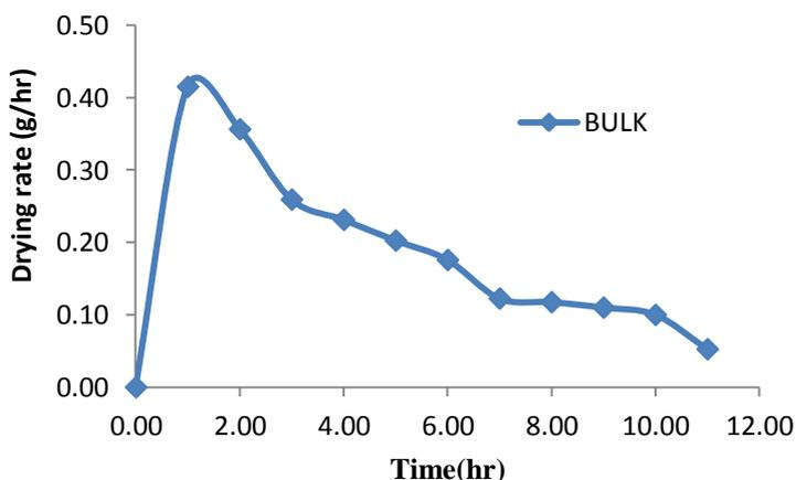
Figure 4: drying rate against drying time for bulk spear grass vegetable
