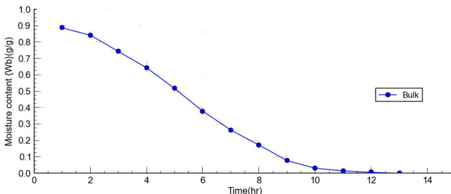
Figure 14: moisture content variation against time of drying the bulk carrot
