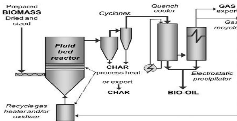
Scheme of the Fast Pyrolysis Process
