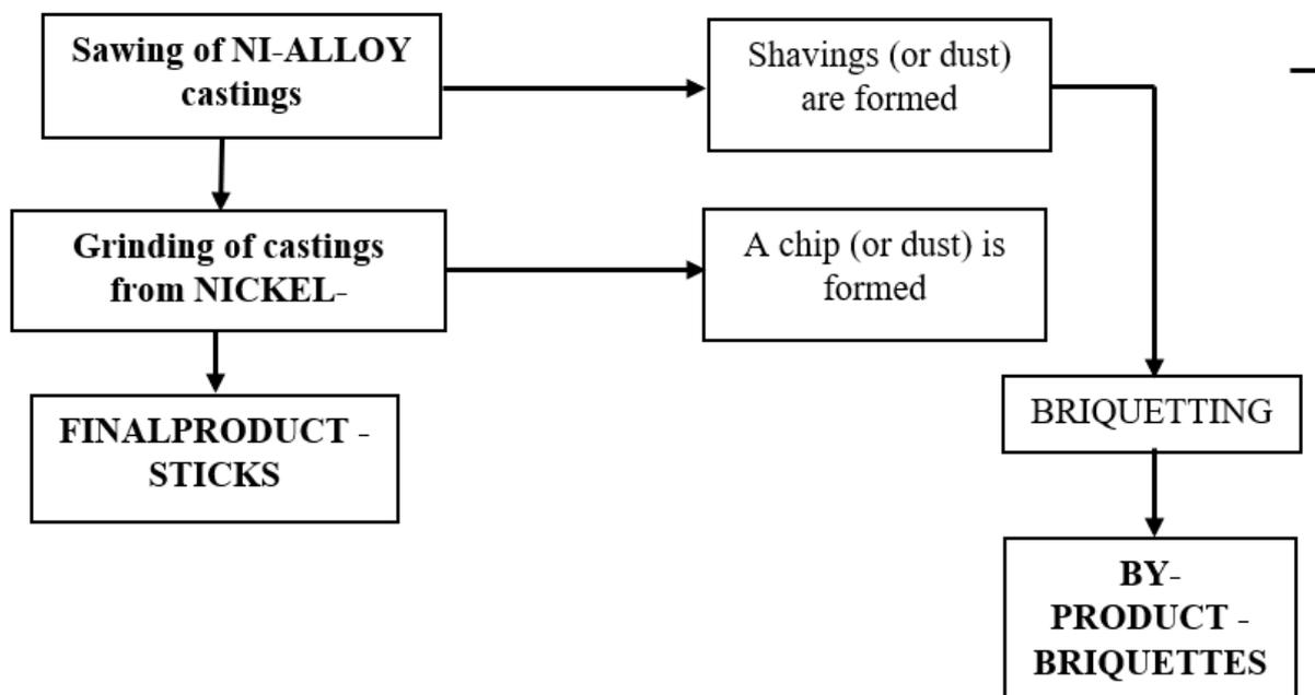
**Picture no 1:** Uniform process - for the purpose of recycling Nickel-alloy powder (source: Own)
