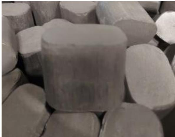
**Picture no 2:** Briquettes - made from Ni-alloy powder
