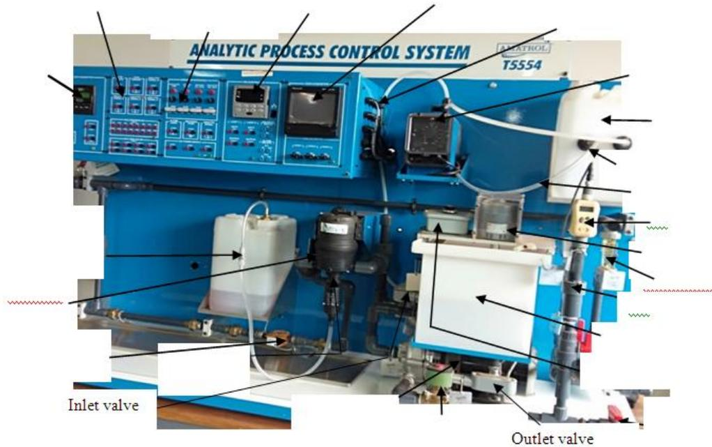
**Figure 1:** The Physical, T5554 Analytical Process Control System<sup>[17]</sup>
