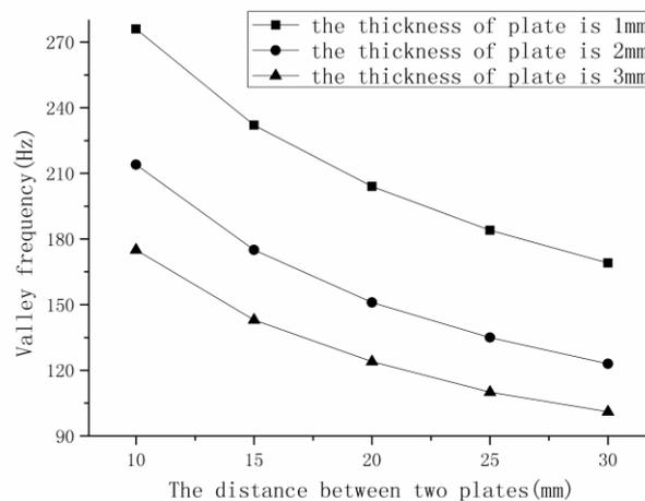
Fig. 12 The curve of valley frequency with different distances between two plates
