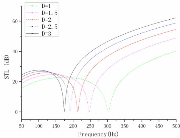
Fig. 9 Sound insulation performance of double-layer plate with different plate thickness
