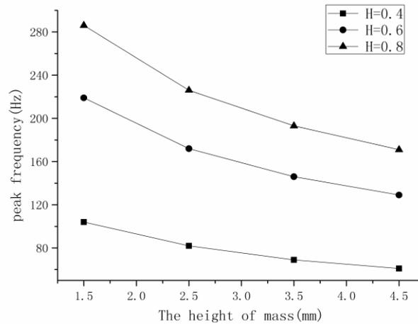
Fig. 8 The curve of peak frequency with different mass blocks
