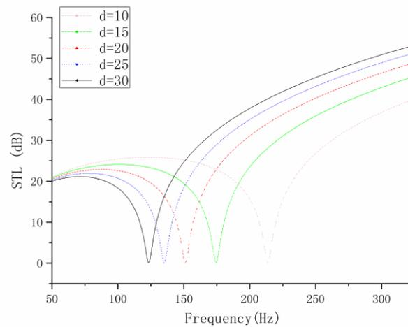
Fig. 11 Sound insulation performance of double-layer plate with different distances between two plates
