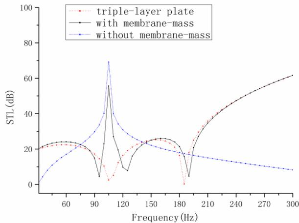
**Fig. 3 Comparison of sound insulation performance of membrane type acoustic metamaterial, cavity triple-layer plate and triple-layer plate with membrane type acoustic metamaterial**
