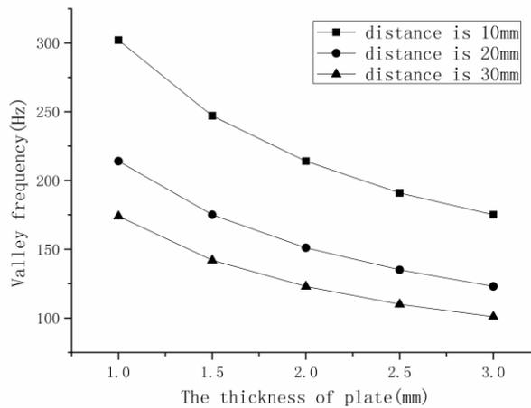
Fig. 10 The curve of valley frequency with different plate thickness
