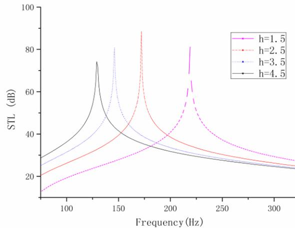
Fig. 7 Sound insulation performance of membrane type acoustic metamaterial with different mass blocks
