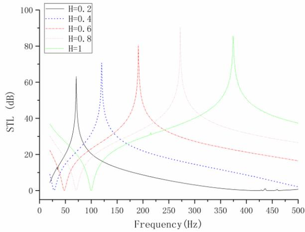
Fig. 4 Sound insulation performance of membrane type acoustic metamaterial with different membrane thickness
