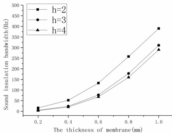
Fig. 6 The curve of sound insulation bandwidth with different membrane thickness
