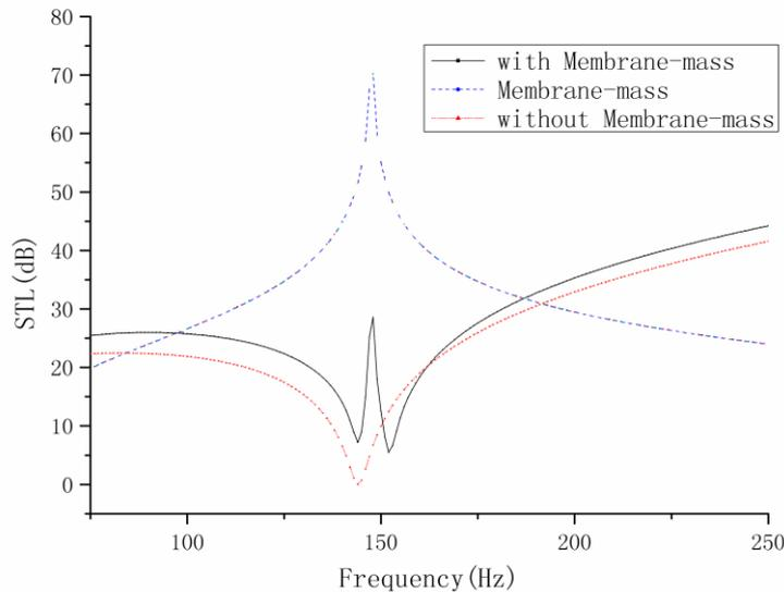
**Fig.2 Comparison of sound insulation performance of membrane-type acoustic metamaterial, cavity double-layer plate and double-layer plate with membrane-type acoustic metamaterial**
