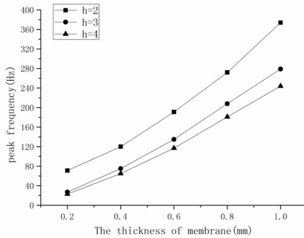
Fig. 5 The curve of peak frequency with different membrane thickness
