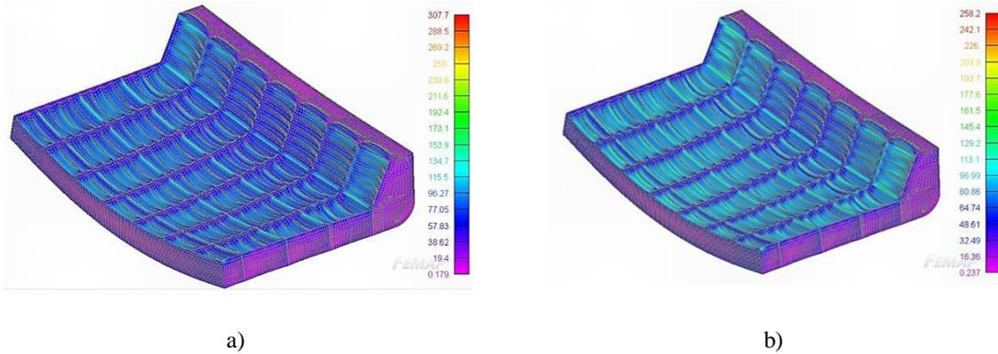
**Figure 11** The case of laying on a wave gap, VonMises voltages on the complete 3D-FEM model
