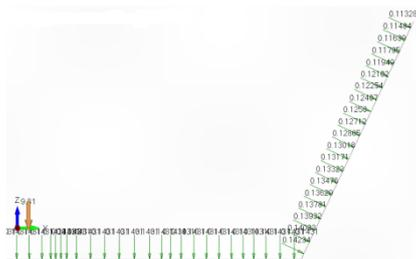
**Figure 5** Distribution of the hydrostatic pressure of the goods on the double shell
