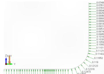
**Figure 6** Distribution of hydrostatic water pressure on the outer shell
