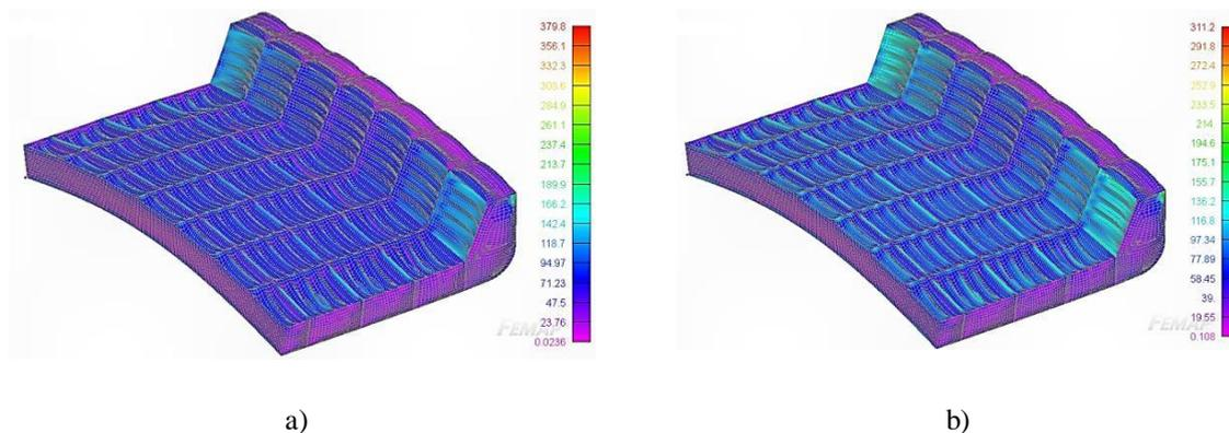
**Figure 13** The case of sitting on the wave ridge, VonMises voltages on the complete 3D-FEM model
