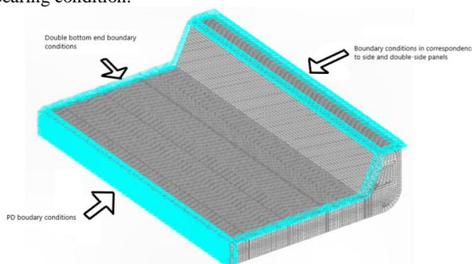
**Figure 4** Edge conditions applied to the 3D-FEM model
