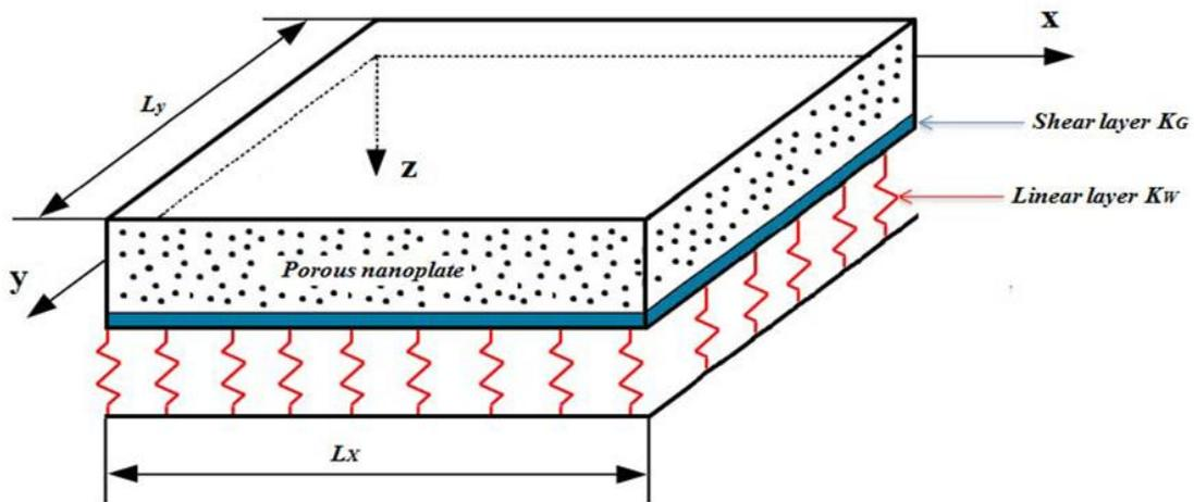
**Figure 1:** Configuration of porous single-layered inhomogeneous nanoplate
