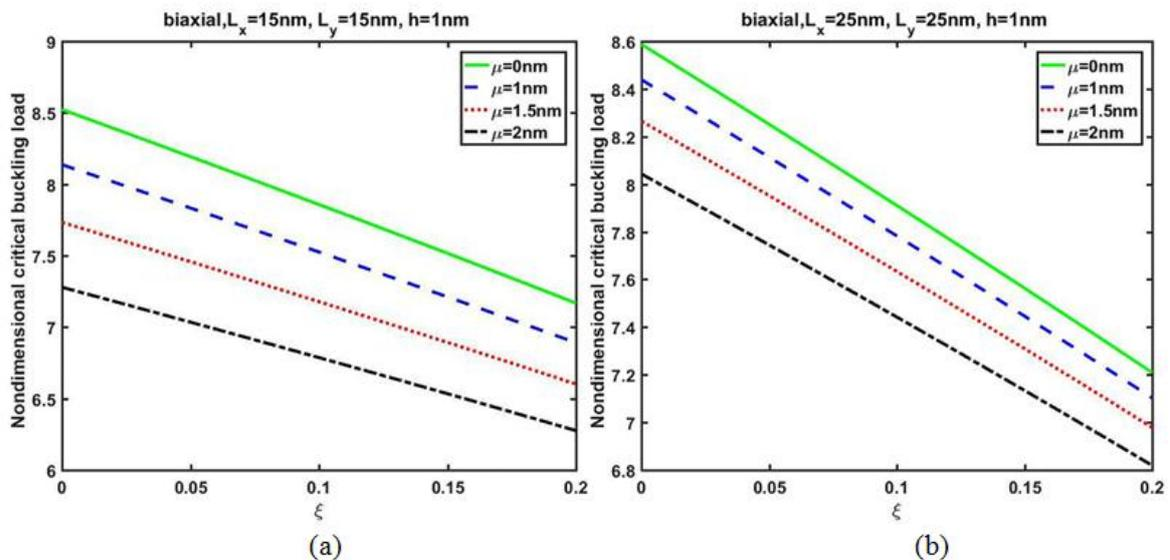
**Figure 2:** Effect of porosity volume fraction on the nondimensional critical buckling load for different nonlocal parameter and biaxial buckling (k=1)
