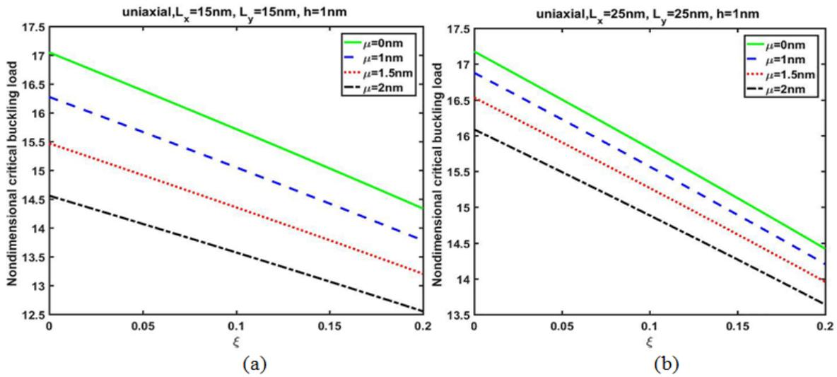
**Figure 3:** Effect of porosity volume fraction on the nondimensional critical buckling load for different nonlocal parameter and uniaxial buckling ( $k=0$ )
