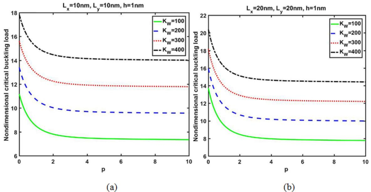
**Figure 4:** Effect of power-law index on the nondimensional critical buckling load for different value of nondimensional Winkler parameter
