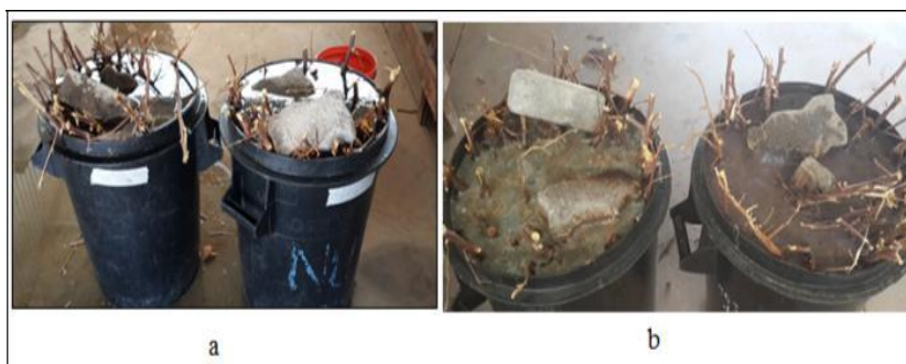
Fig 2.1. Showing natural water retting of cotton stalks at initial (a) and after three weeks (b) After the retting process the cotton stalks were subject to manual decortication using a rubber coated hammer to avoid damage to the cotton stalk fibres as shown in Fig 2.2. There after the cotton stalk fibres were cleaned and combed to remove any adhering dirt particles [15].
