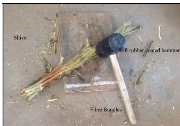
Fig 2.2. Mechanical decortication process in the extraction of cotton stalk fibres [15]
