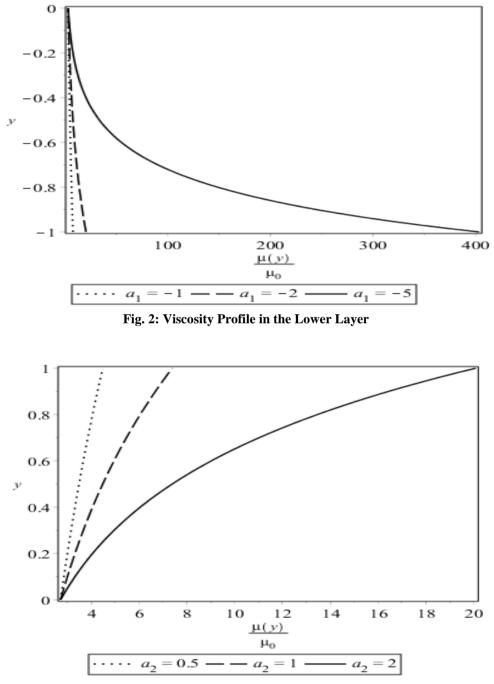
Fig. 3: Viscosity Profile in the Upper Layer
