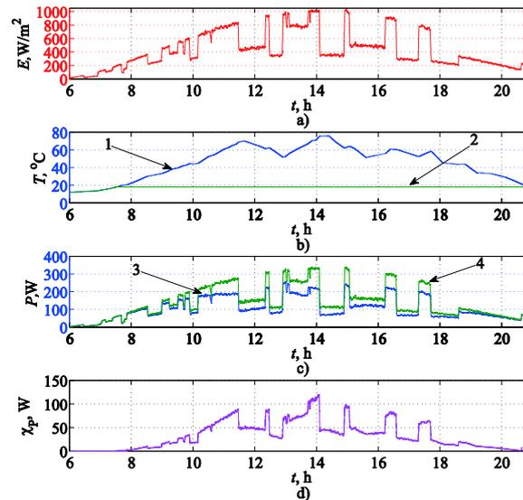
**Figure 5 Solar power flux (a), temperature of PV modules during a slightly windy day without forced cooling (b-1), temperature of PV modules during a slightly windy day with forced cooling to 18°C (b-2), instantaneous power of solar power plant without forced cooling (c-3), instantaneous power of solar power plant with forced cooling to 18°C (c-4), instantaneous difference of output power (d).**
