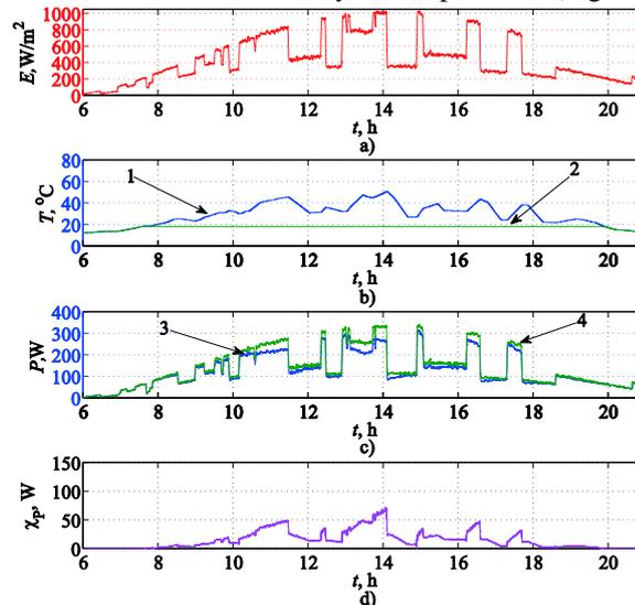
**Figure 6** Solar power flux (a), temperature of PV modules during windy day without forced cooling (b-1), temperature of PV modules during windy day with forced cooling to 18°C (b-2), instantaneous power of solar power plant without forced cooling (c-3), instantaneous power of solar power plant with forced cooling to 18°C (c-4), instantaneous difference of output power (d).
