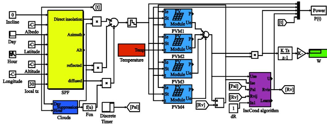
Figure 3 Matlab/Simulink model with temperature block
