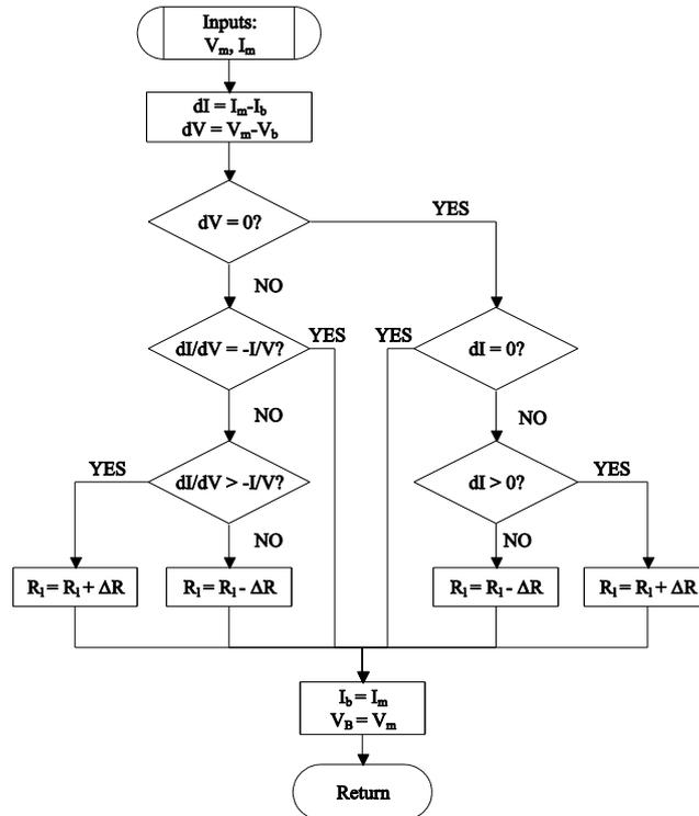
Figure 4 The flowchart of IncCond algorithm, implemented in the model of solar power plant
