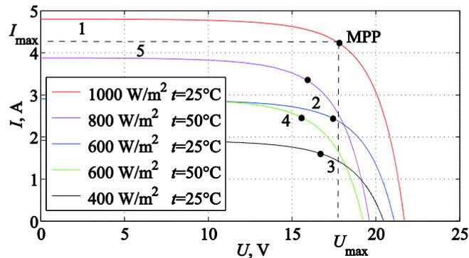
Figure 1 MPP at different SPF and temperatures [6]
