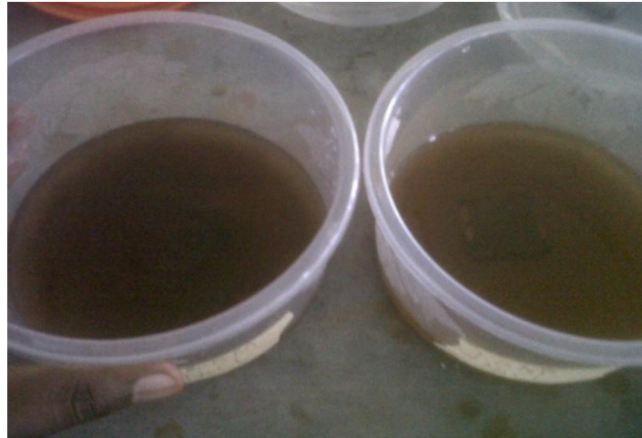
Fig. 6: Brownish suspension in NaCl solution of 0.5M and 1.0M concentration
