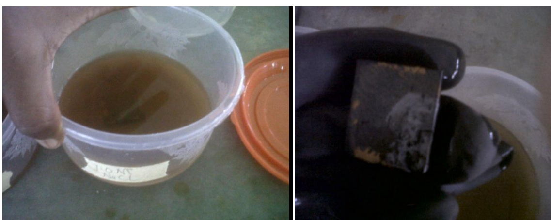
Fig. 3: Corrosion product formed on coupon
