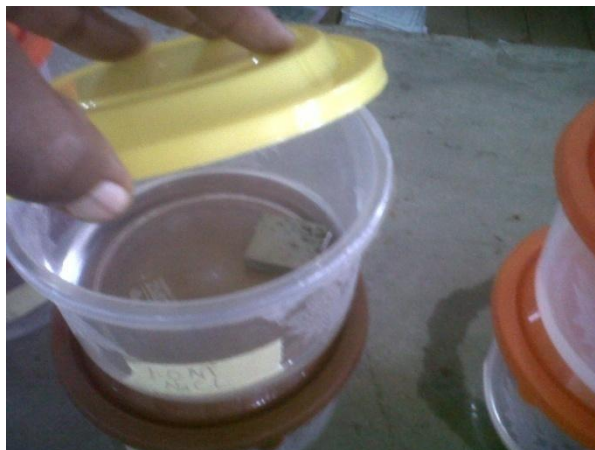
Fig. 2: Immersion of coupons and setup
