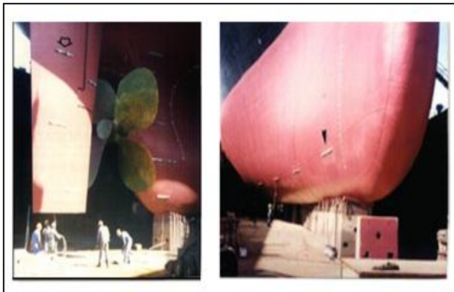
Figure 2 – Aspects of galvanic anodes disposal in the stern and the bow
