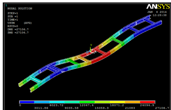
Fig: Displacement vector sum of dof solution
