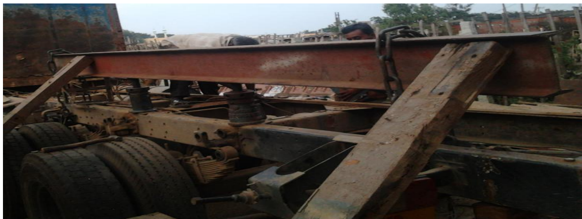
Fig : chassis deformed due to heavy weights
