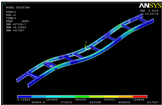
Fig: vonmises stress of the chassis
