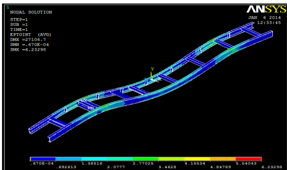
Fig: Total mechanical strain intensity
