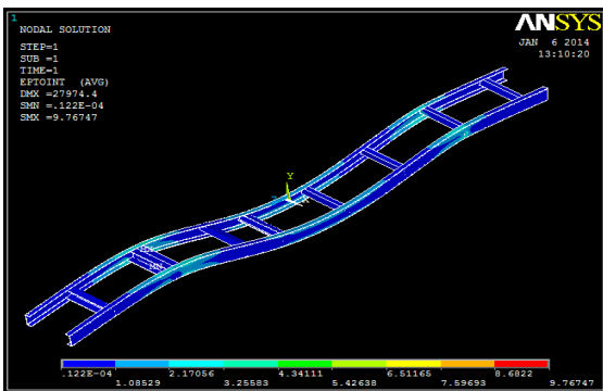
Fig: Total mechanical strain intensity
