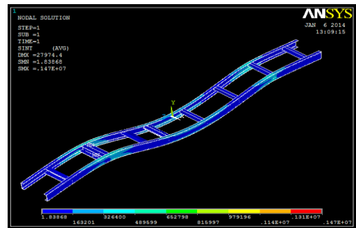
fig: stress intensity of the chassis
