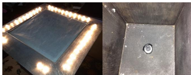
Fig. 3 Multi-touch table outside and inside view.
