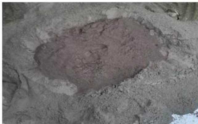
Fig.3: Waste paper sludge ash added to cement for blending
