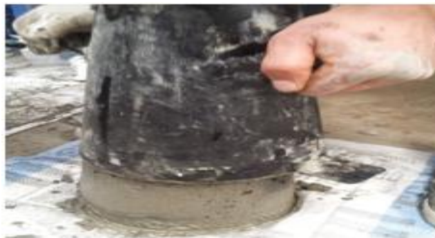
Fig.4: Slump cone being removed slowly.
