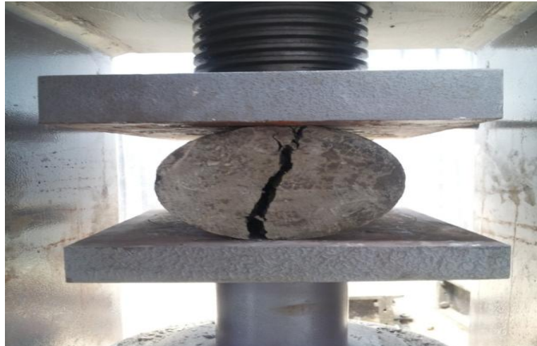
Fig. 6. Cylinder specimen failing in splitting cylinder test
