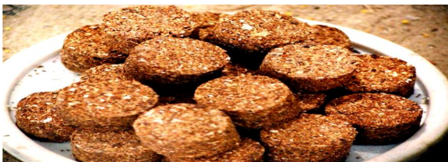
Plate 4: Briquettes produced from maize cob and banana peel binder
