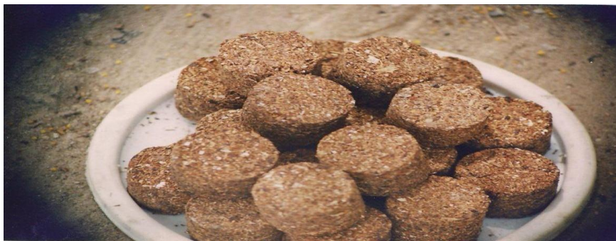
Plate 3: Briquettes produced from maize cob and cassava peel gel binder
