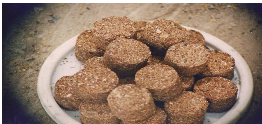
Plate 6: Briquettes produced from sugarcane baggasse and banana peel binder
