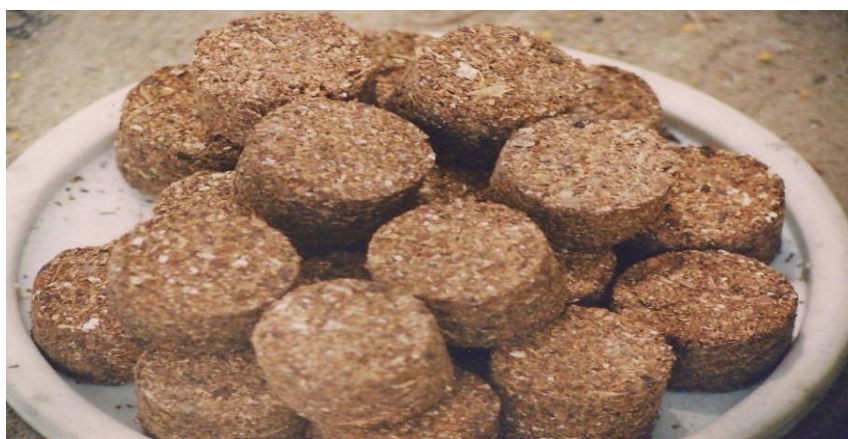
Plate 5: Briquettes produced from sugarcane baggasse and cassava peel gel binder
