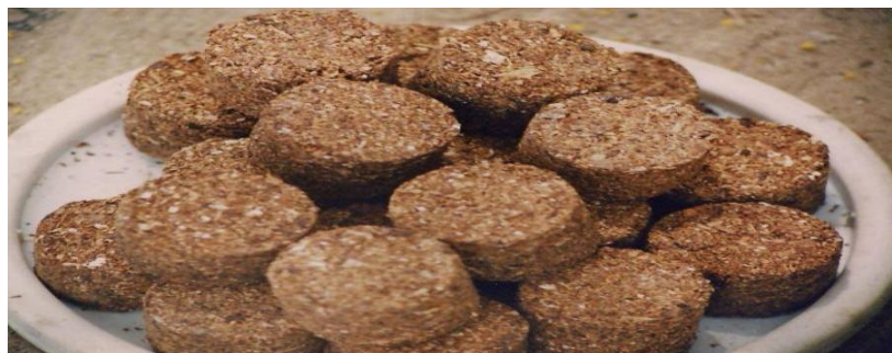
Plate 2: Briquettes produced from rice husk and banana peel binder
