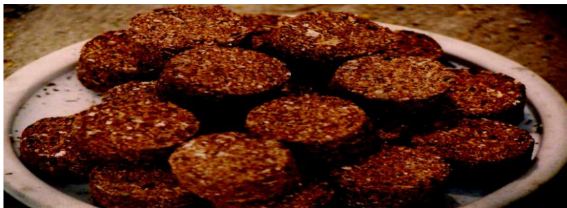
Plate 7: Briquettes produced from groundnut shell and cassava peel gel binder
