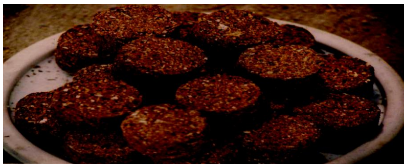
Plate 8: Briquettes produced from groundnut shell and banana peel binder
