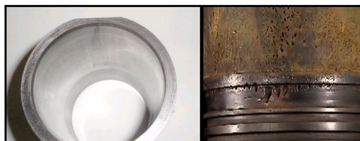
Fig. 5. Liner damages cause by wall cracking, corrosion, cavitation erosion and excessive wear [12]
