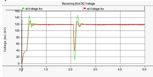
Figure 7.2 (i) DC voltage waveform at the time of LL-G fault, with and without STATCOM
