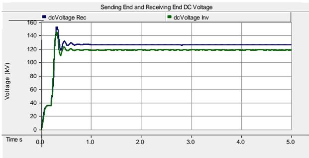
Figure7.1 (a) DC voltage waveform at the time of line charging , without STATCOM
