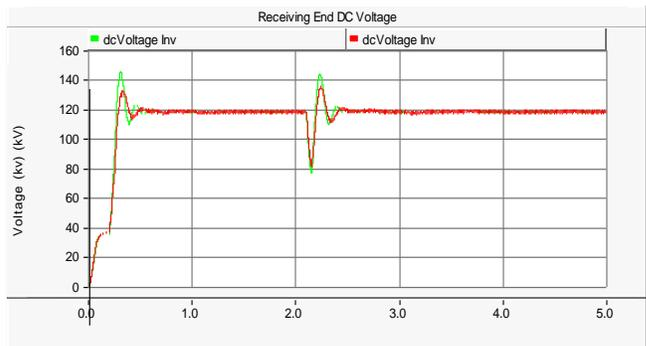
Figure 7.2(c) DC voltage waveform at the time of L-G fault, with and without STATCOM
