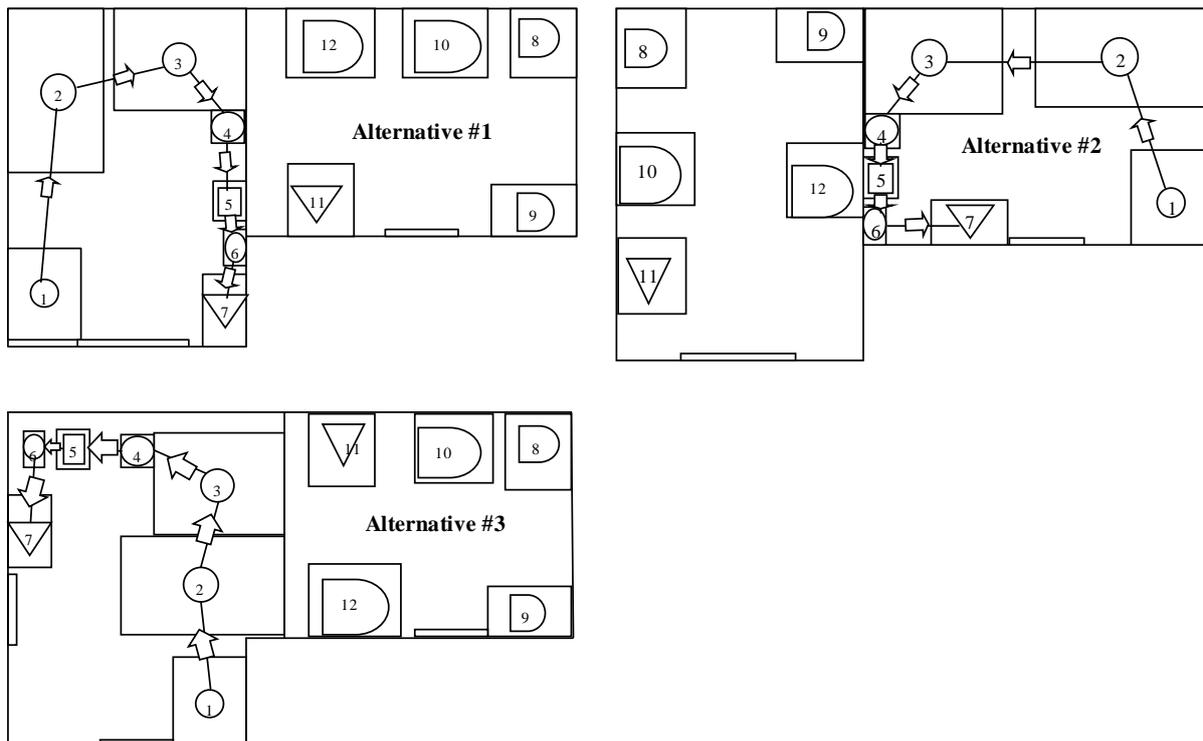
Figure 4 The alternative facility layout for germinate brown rice mill.
