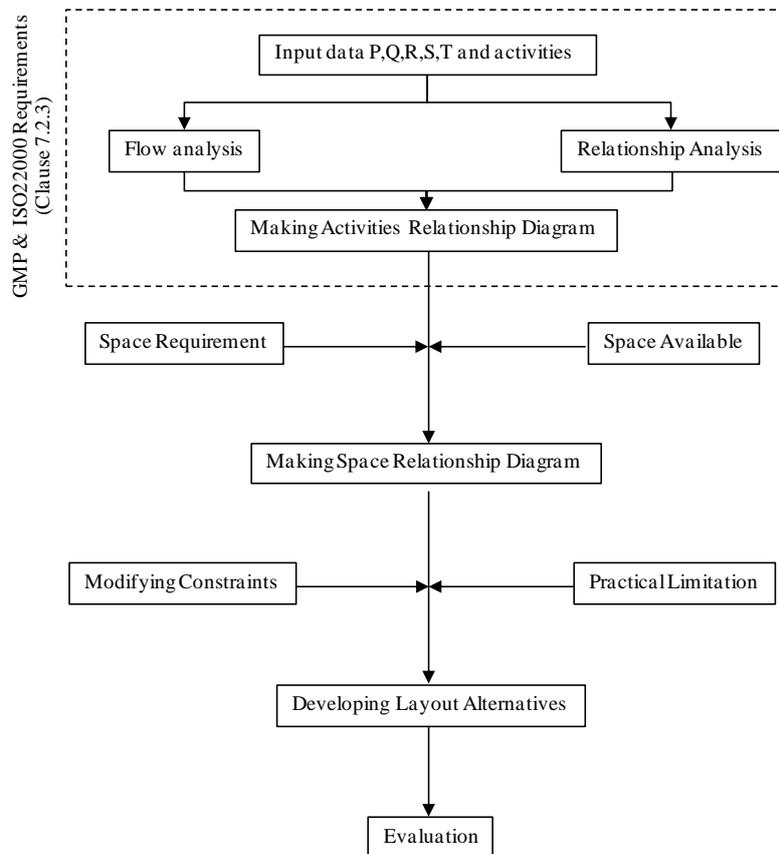
**Figure 1** Systematic Layout Planning with GMP and ISO22000 requirements.
