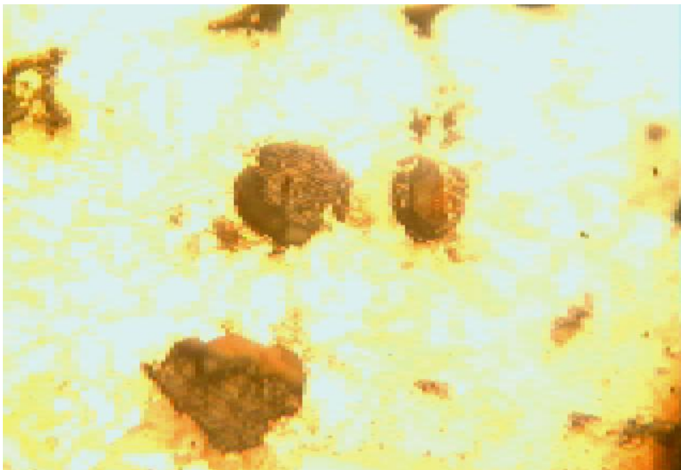
Plate 5: Microstructure of ductile iron austenitized at 950 °C austempered in jatropha seed oil at 250 °C for 4 hrs, showing graphite nodules (black) in austenite matrix; (x400)
