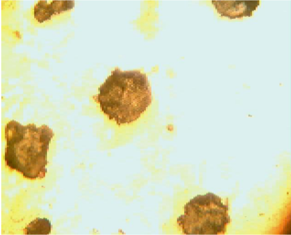
Plate 6: Microstructure of ductile iron austenitized at 950 °C austempered in jatropha seed oil at 250 °C for 5 hrs, showing graphite nodules (black) in ausferrite matrix; (x400)
