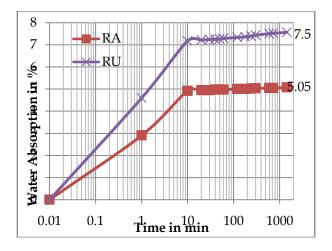
Fig. 2 water absorption vs logarithmic time
