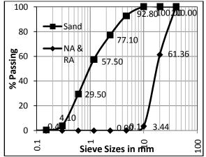
Fig. 1 Grading Curve of Fine and Coarse Aggregate
