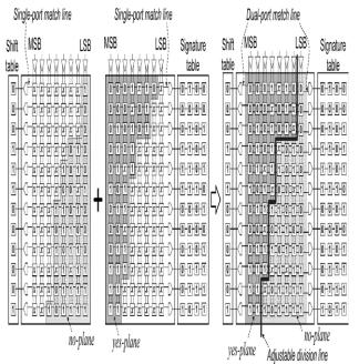
Fig .2. The design Concept of the proposed dual-port TCAM.
