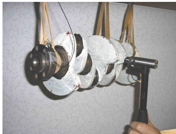
Fig. 9. The accelerometer to the left, the impact hammer to the right
