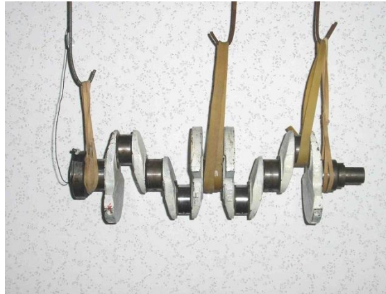
Fig.11. Crankshaft suspended on elastic cables
