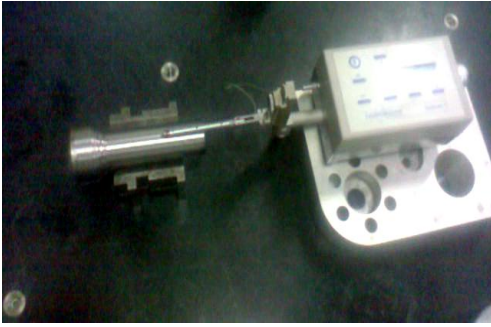
Figure 4: Photographic view of TR 200 surface roughness tester
