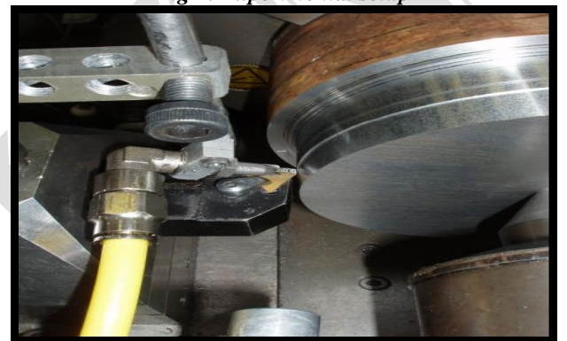
Fig3: Machining using Mist Cooling
