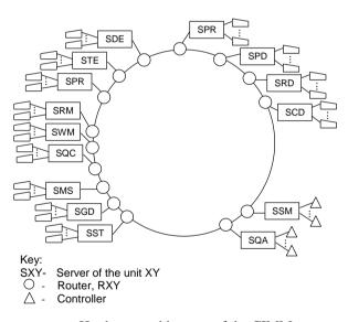
Figure 1. Hardware architecture of the CIMM system
