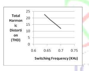
Fig.6 Switching Frequency Vs THD
