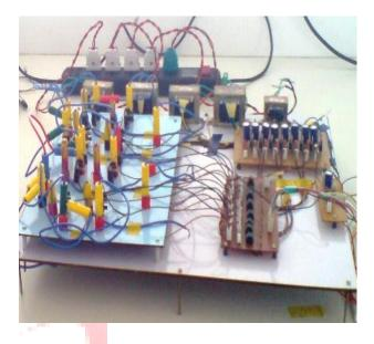
Fig.7. Photograph of the prototype of seven-level inverter
