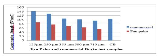
Effect of particle size on compressive strength values for fan palm and commercial brake pads
