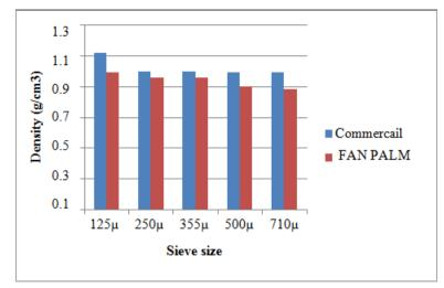
Figure 4.3: Effect of particle size on density of periwinkle and fan palm shel
